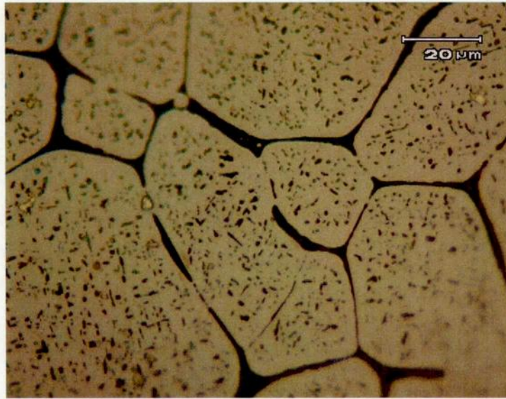
Fig. 2.3.72. Metallographic appearance of the hydride of Zr-Gd alloy (Zr : Gd = 10 : 1, H/M=1.93).
