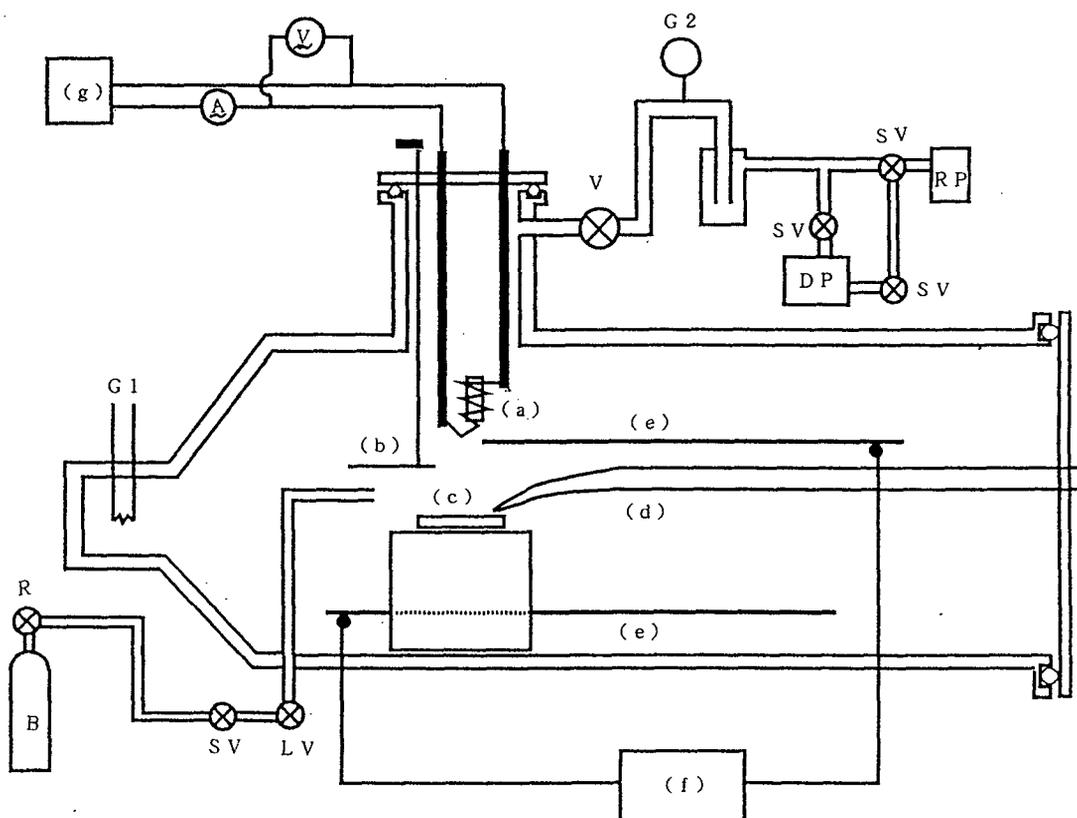
Fig. 1 Schematic drawing of the apparatus used for the reactive vapor deposition. (a); W filament where  $\alpha$ -Mn flakes are placed, (b); shutter, (c); substrate, (d); thermocouple, (e); Ta electrode for glow discharge, (f); neon transformer, (g); electric power supply, A; ammeter, V; voltmeter, G1; pirani gauge, G2; ionization gauge, LV; leak valve, SV; stop valve, R; regulator for  $N_2$  gas cylinder, V; main valve, and conductance valve, DP; oil diffusion pump, RP; rotary pump.
