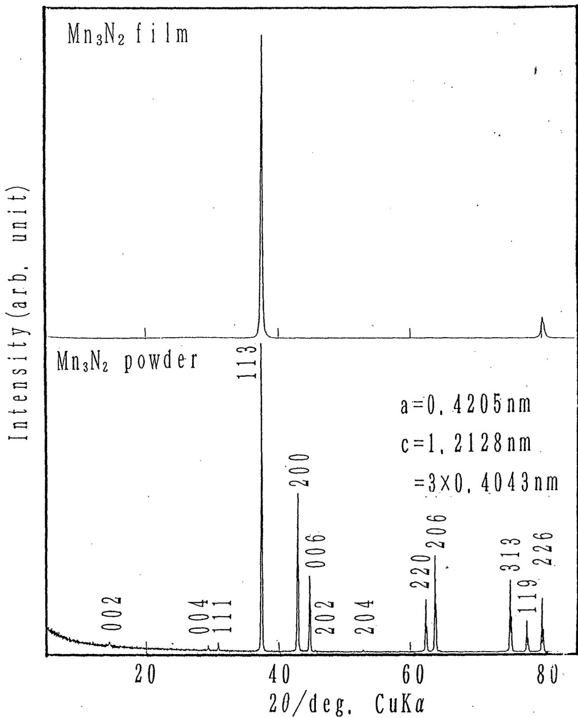
Fig. 3 X-ray diffraction patterns for the Mn<sub>3</sub>N<sub>2</sub> film deposited at  $E_p$  of 240W and  $p_N$  of 2.6Pa and Mn<sub>3</sub>N<sub>2</sub> powder obtained successively firing  $\alpha$ -Mn powder at 873K in NH<sub>3</sub> and H<sub>2</sub> flow.
