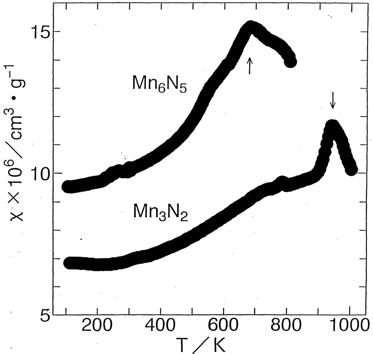
Fig. 2. Temperature dependence of magnetic susceptibility for  $\text{Mn}_6\text{N}_5$  and  $\text{Mn}_3\text{N}_2$ .
