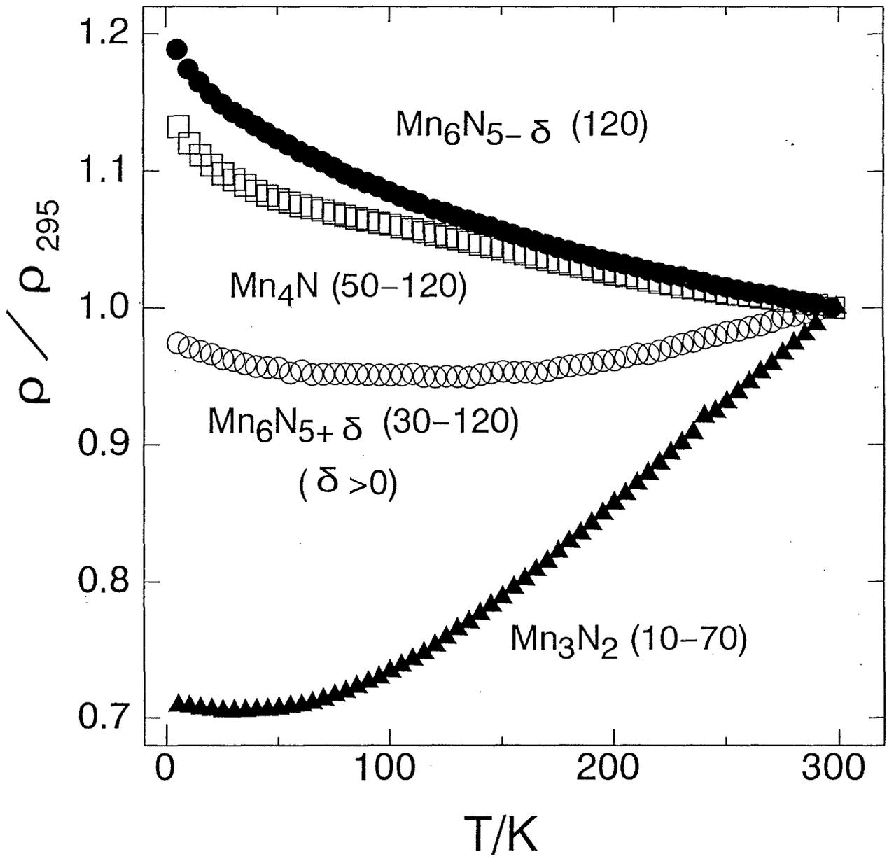
Fig. 7 Temperature dependence of electrical resistivity ratios ( $\rho/\rho_{295}$ ) for  $MnN_y$  films.  $\rho_{295}$  denotes the electrical resistivity at 295K. The value of  $\rho_{295}/\mu\Omega m$  for each samples is designated in parentheses.
