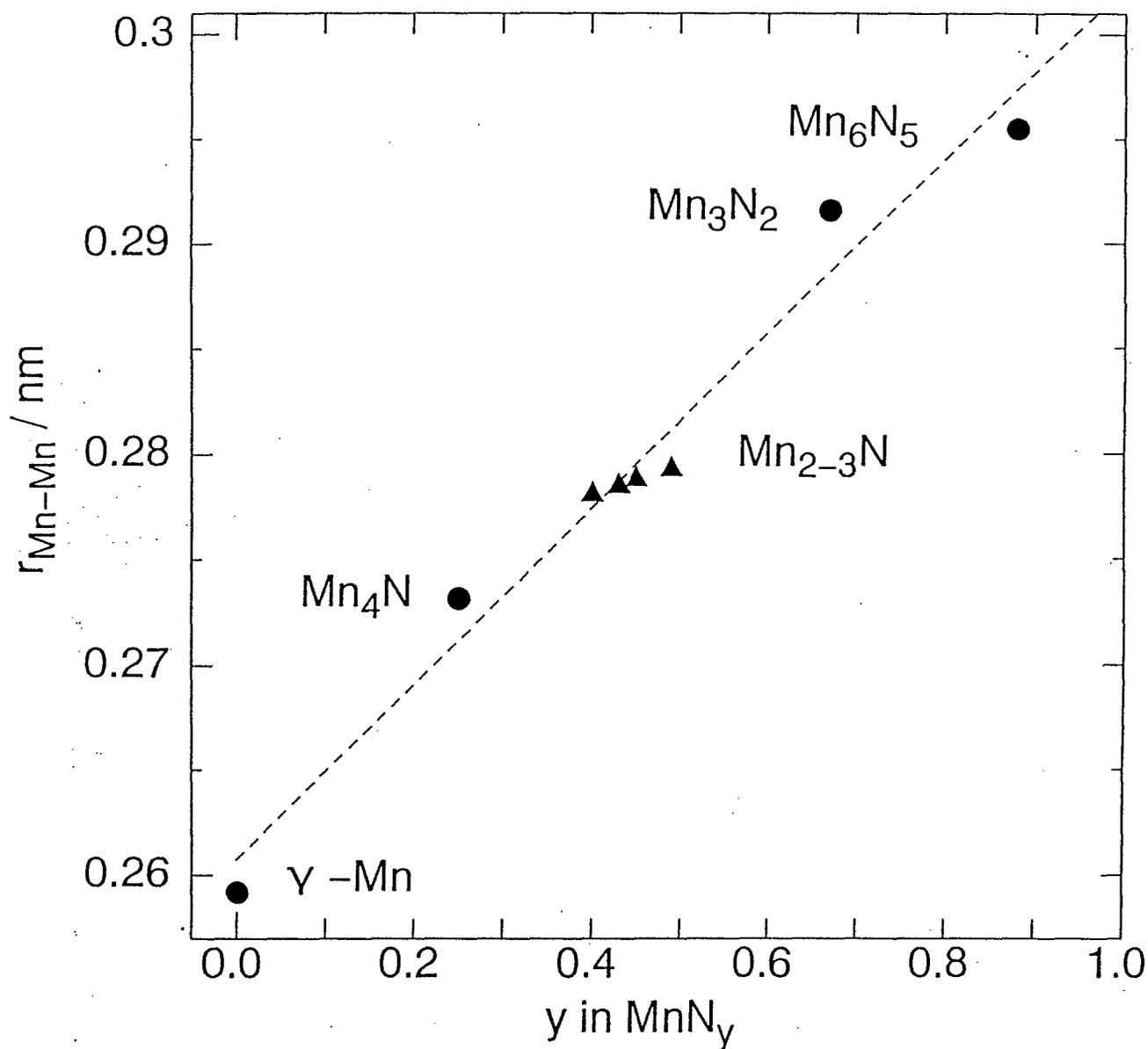
Fig. 3. The relation between nitrogen content  $y$  and the shortest Mn-Mn distance,  $r_{\text{Mn-Mn}}$ . Closed circle denotes that Mn has fcc or fct lattice, and closed triangle denotes that Mn takes hcp lattice. The values of  $r_{\text{Mn-Mn}}$  correspond to the shortest Mn-Mn distance in a plane parallel to the  $c$ -axis. The dashed line indicates the line obtained by least square fitting between  $y$  and  $r_{\text{Mn-Mn}}$  with 0.986 of correlation coefficient.
