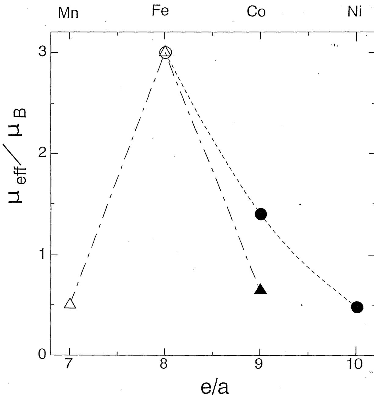
Fig. 7. The relation between the formal valence electron number per a metal atom,  $e/a$  and the effective magnetic moment per a metal atom,  $\mu_{\text{eff}}$  for  $M_{2-3}N$  ( $\circ$  [19],  $\bullet$ ; present results) and  $M_2N$  ( $\triangle$  [19],  $\blacktriangle$ ; present results). Dot-dashed line and dotted curves show that  $\mu_{\text{eff}}$  of  $M_2N$  and  $M_{2-3}N$ , respectively, exhibit the behavior such as Slater-Pauling curve observed in 3d metal alloys.
