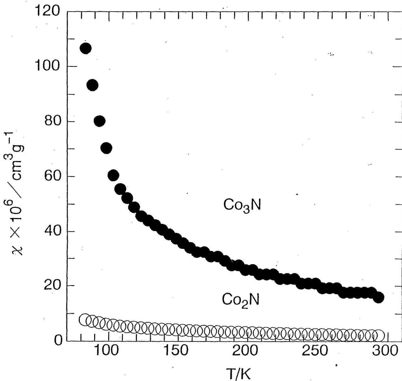
Fig. 4. Temperature dependence of magnetic susceptibility for  $\text{Co}_3\text{N}$  and  $\text{Co}_2\text{N}$ .
