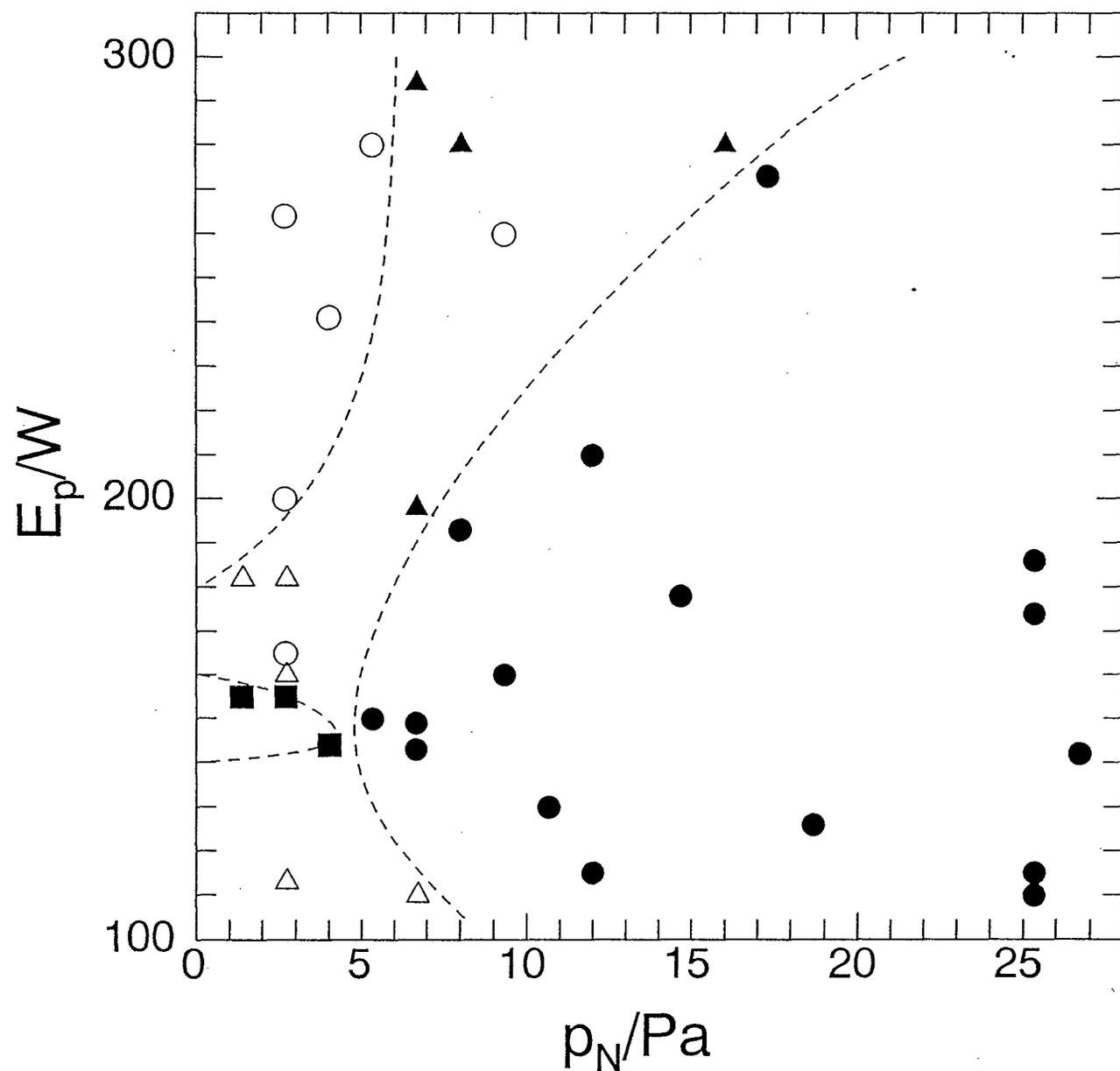
Fig. 6 The relation among crystal phase in products, nitrogen gas pressure during deposition ( $p_N$ ) and electric power applied to W filament ( $E_p$ ).
