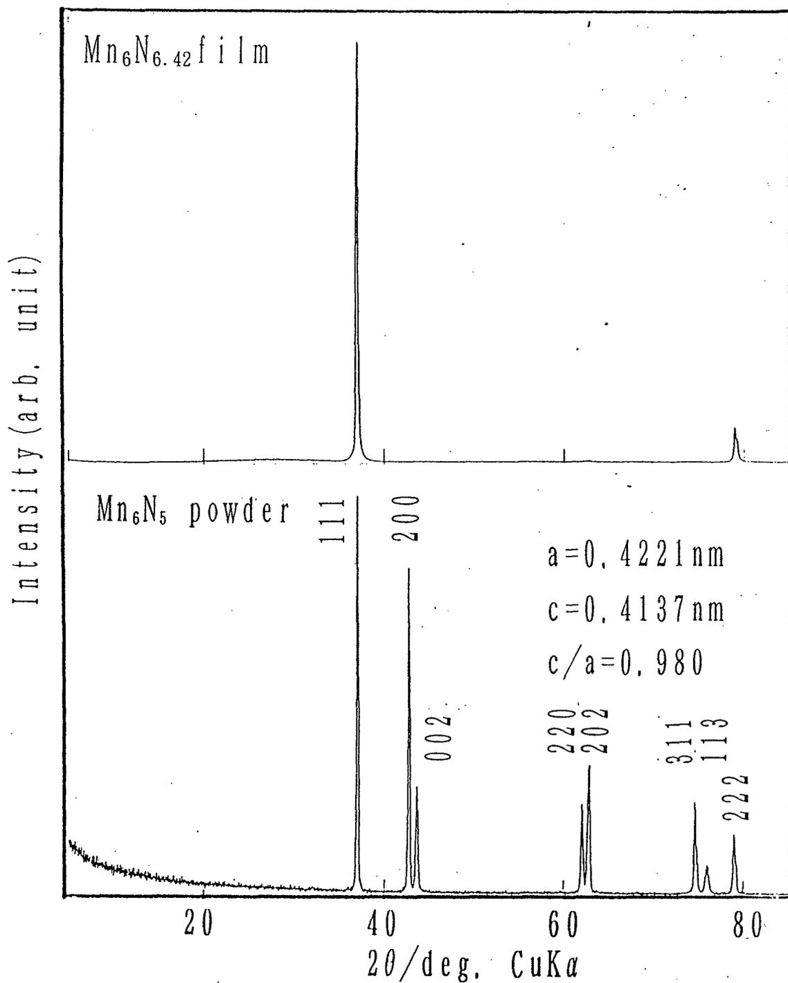
Fig. 4 X-ray diffraction patterns for the Mn<sub>6</sub>N<sub>6.42</sub> film deposited at  $E_p$  of 186W and  $p_N$  of 25Pa and (b) Mn<sub>6</sub>N<sub>5</sub> powder obtained firing  $\alpha$ -Mn powder at 873K in NH<sub>3</sub> flow.
