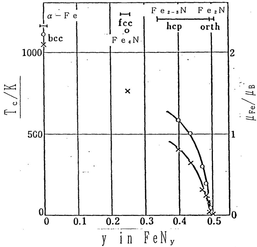
Fig. 3. Plots of the magnetic moments ( $\mu_{\text{Fe}}$ : O) and Curie temperature ( $T_c$ : x) against the nitrogen contents of  $\text{FeN}_y$  ( $y \leq 0.5$ ) [4].
