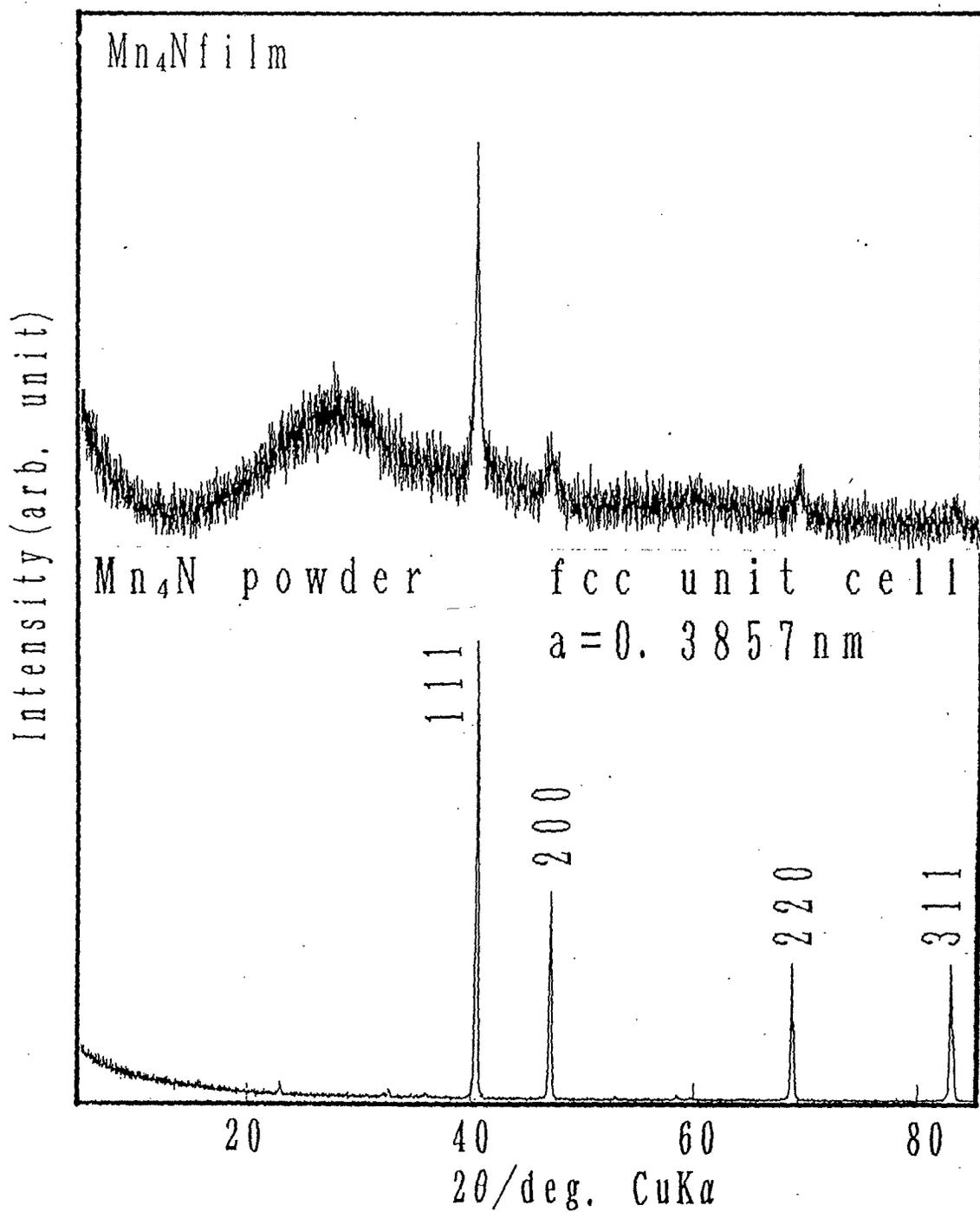
Fig. 2 X-ray diffraction patterns for the Mn<sub>4</sub>N film deposited at  $E_p$  of 155W and  $p_N$  of 1.3Pa, and Mn<sub>4</sub>N powder obtained successively firing  $\alpha$ -Mn powder at 1073K in N<sub>2</sub> and H<sub>2</sub> flow.
