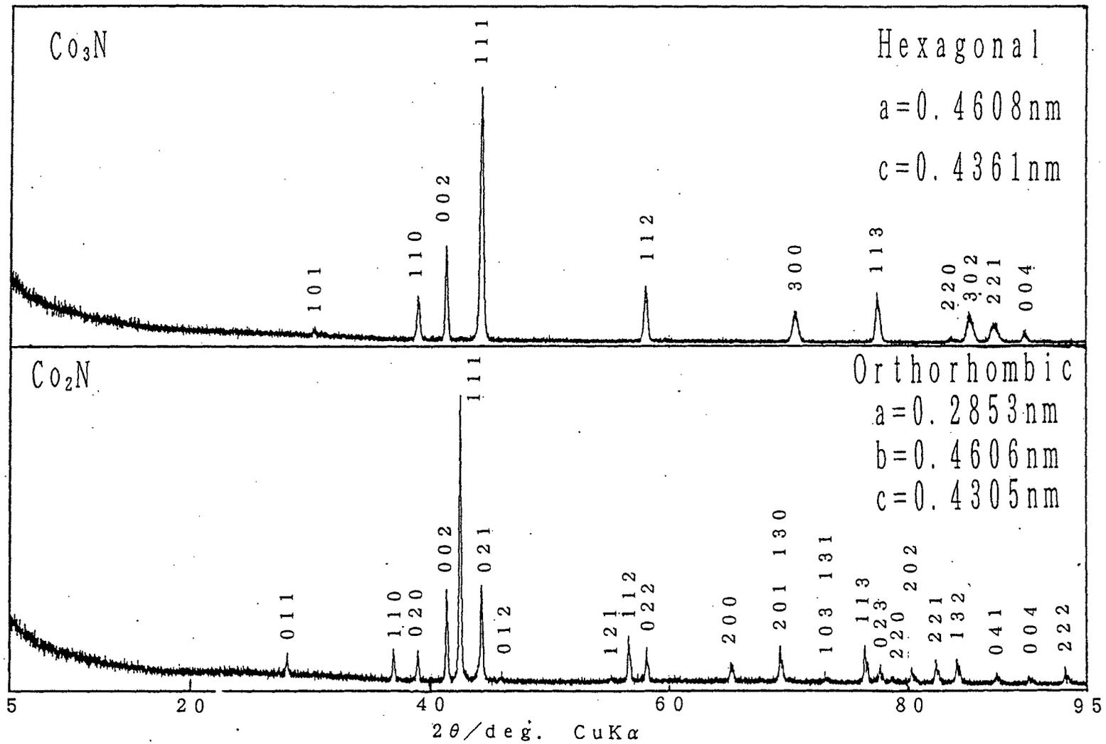
Fig. 1. X-ray diffraction patterns of Co<sub>3</sub>N and Co<sub>2</sub>N.
