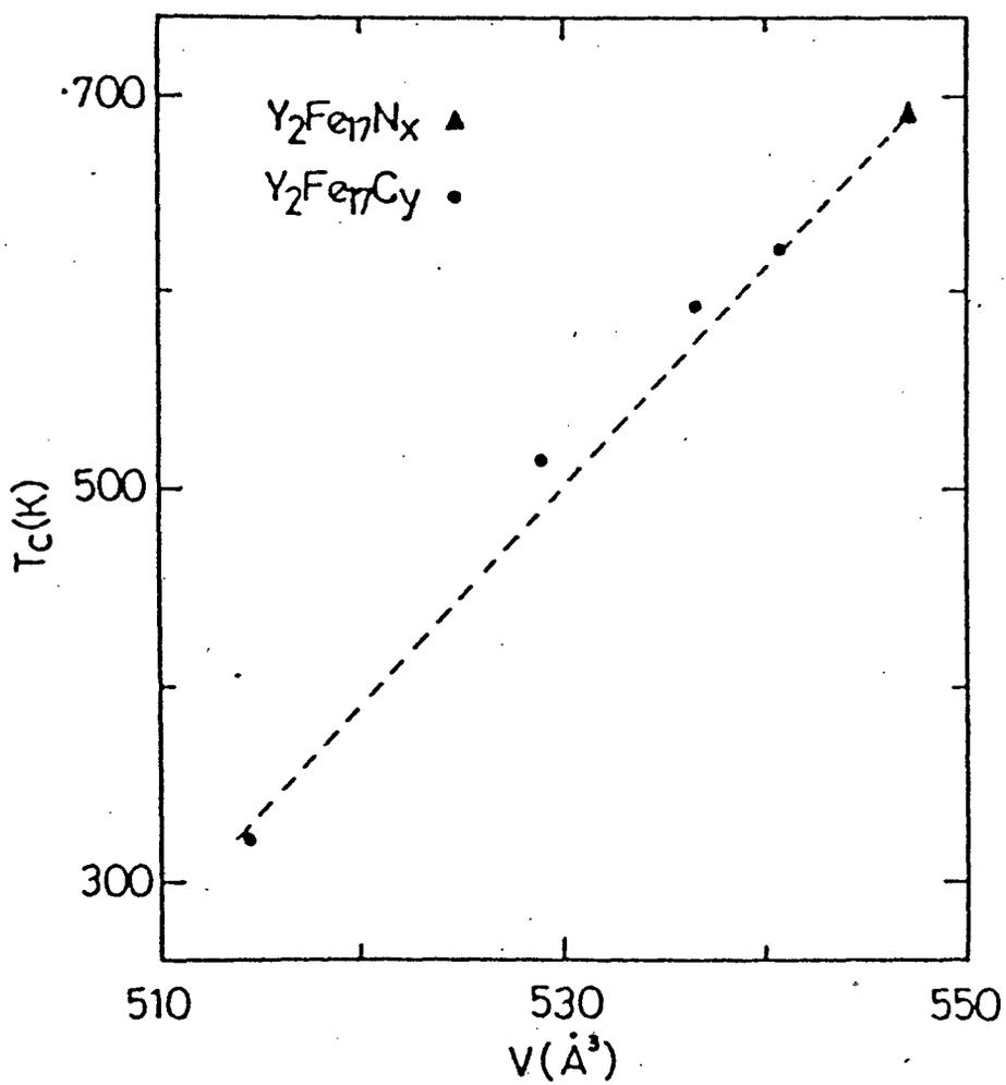
Fig. 2. Volume ( $V$ ) dependence of Curie temperature ( $T_c$ ) of  $\text{Y}_2\text{Fe}_{17}\text{N}_x$  ( $\blacktriangle$ ) and  $\text{Y}_2\text{Fe}_{17}\text{C}_y$  ( $\bullet$ ) [21]. The broken line represents the volume dependence of  $\text{Y}_2\text{Fe}_{17}$ .
