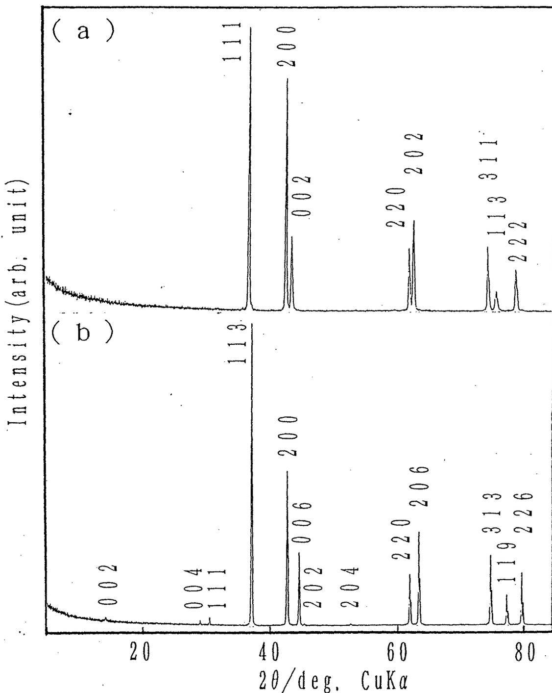
Fig. 1. Powder X-ray diffraction patterns of  $Mn_6N_5$  (a) and  $Mn_3N_2$  (b). In (a), all diffraction peaks were indexed as Mn taking fct cell ;  $a=0.4221\text{nm}$ ,  $c=0.4137\text{nm}$ ,  $c/a=0.980$ . In (b), all diffraction peaks were indexed as Mn taking three fold fct cell along c-axis direction ;  $a=0.4205\text{nm}$ ,  $c=1.2128\text{nm}$ ,  $c/a=0.961$ .
