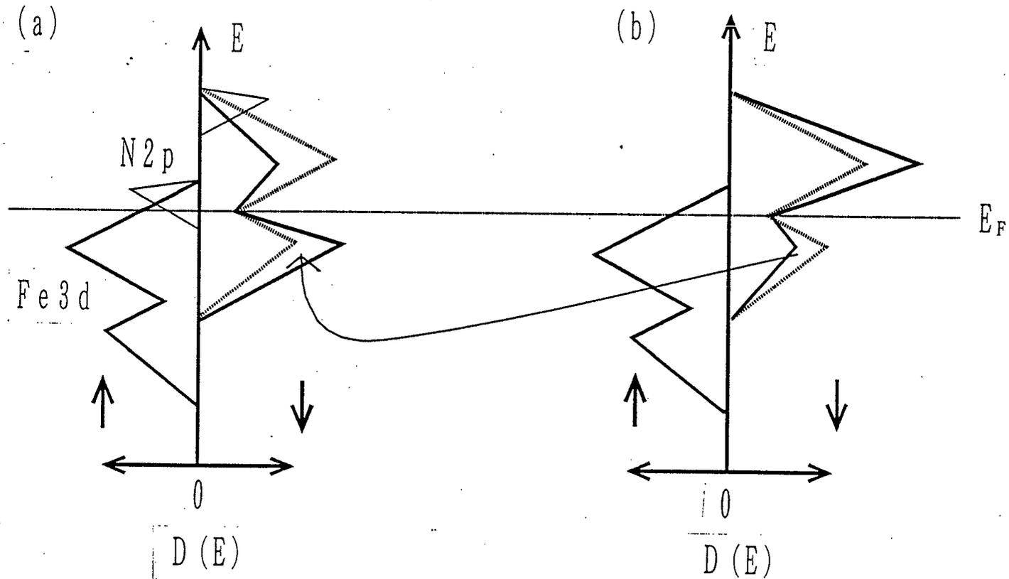
Fig. 6. The local densities of states ( $D(E)$ ) of N 2p band and Fe 3d bands in  $\text{Fe}_4\text{N}$  at the face center positions (Fe(2)) (a), and at the cube corner ones (Fe(1)) (b) [31].  $D(E)$  of Fe(1) and Fe(2) atoms are changed from dotted lines to solid ones with the inclusion of N atoms, and the electrons of down spin states are then transferred from Fe(1) 3d bands to Fe(2) ones. As a result,  $\mu_{\text{Fe}}$  of a Fe(1) atom is raised, while that of a Fe(2) atom is lowered.
