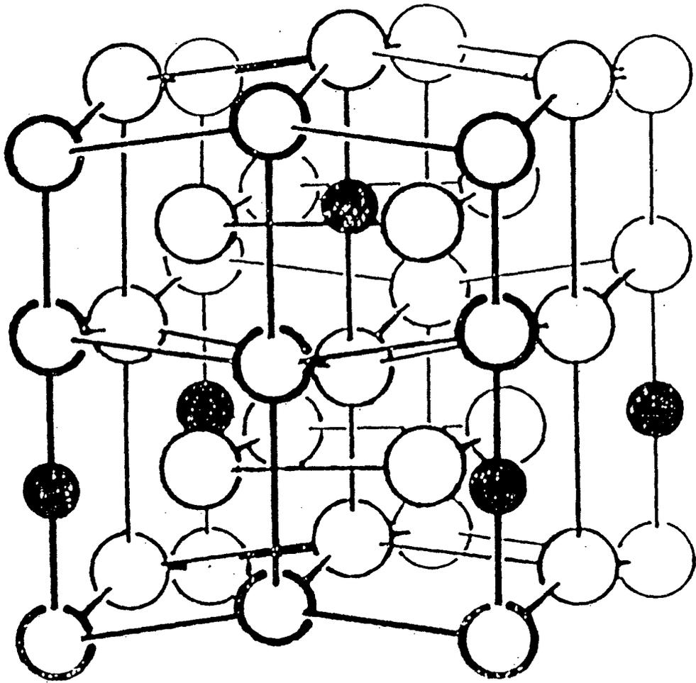
Fig. 4. Crystal structure of  $\text{Fe}_{16}\text{N}_2$  [25]. Open and closed circles denotes Fe and N atoms, respectively.
