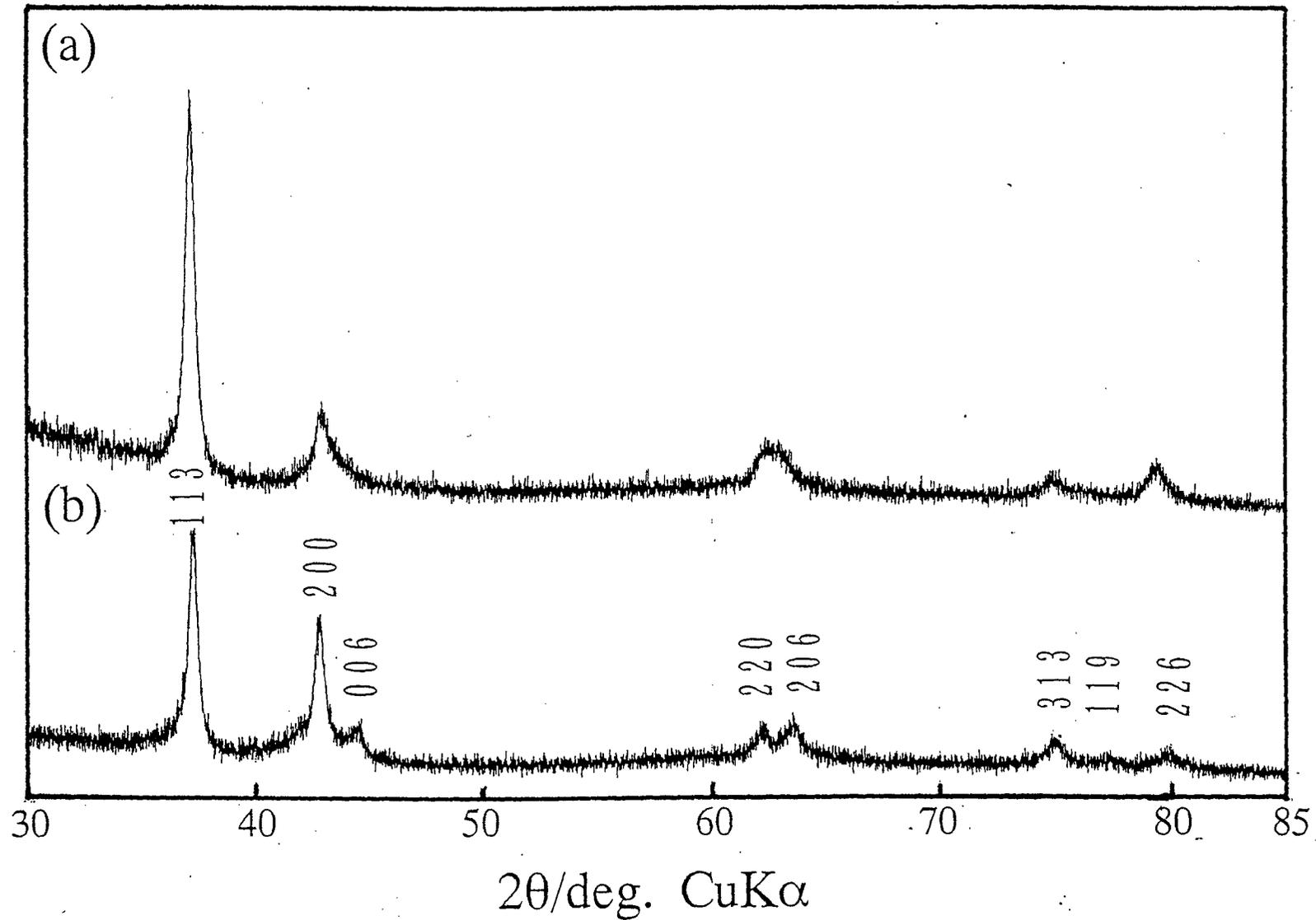
Fig. 5 X-ray diffraction patterns for the  $\text{MnN}_{0.64}$  film deposited at  $E_p$  of 143W and  $p_N$  of 6.5Pa (a) and  $\text{Mn}_3\text{N}_2$  powder deposited at  $E_p$  of 240W and  $p_N$  of 2.6Pa (b).
