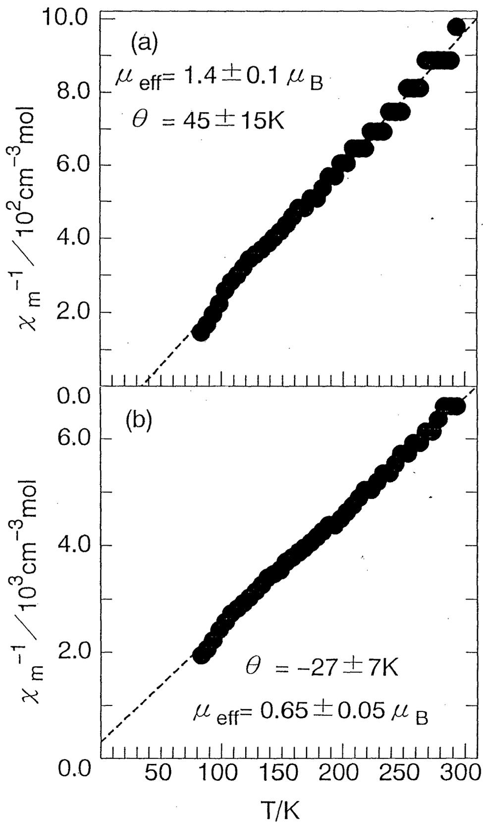
Fig. 5. Temperature dependence of inverse molar susceptibility for  $\text{Co}_3\text{N}$  (a) and  $\text{Co}_2\text{N}$  (b). Weiss temperature,  $\theta$  and the effective magnetic moment per a metal atom,  $\mu_{\text{eff}}$  were described in this figure.
