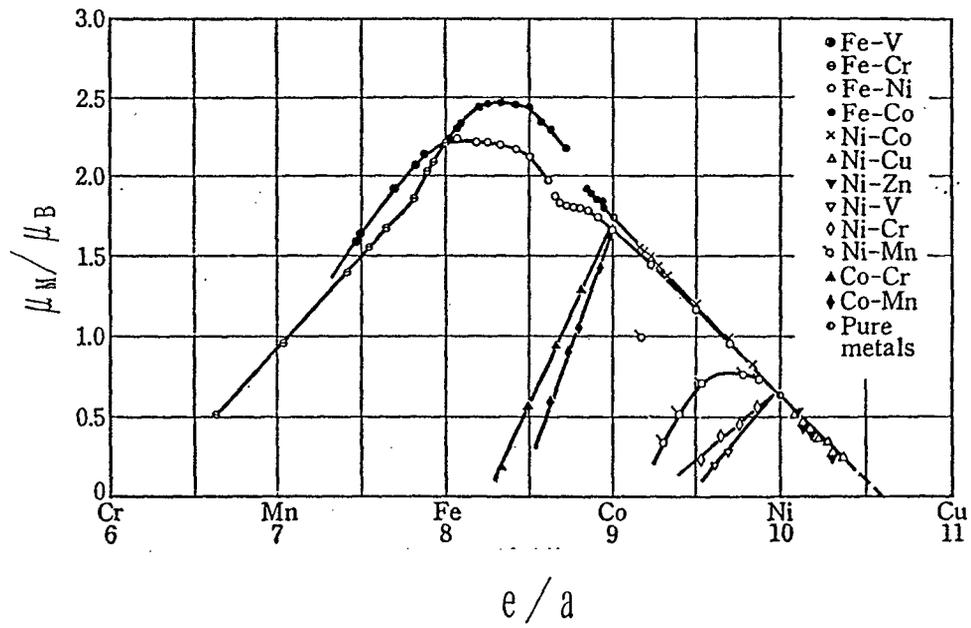
Fig. 8. The relation between magnetic moment per a metal atom ( $\mu_M$ ) and number of valence electrons per a M atom ( $e/a$ ) in 3d metals and their alloys "Slater-Pauling curves" [22].
