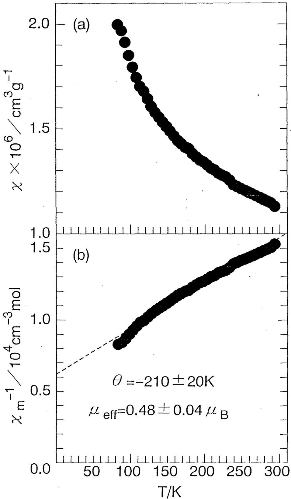
Fig. 6. Temperature dependence of magnetic susceptibility (a) and inverse molar susceptibility (b) for  $\text{Ni}_3\text{N}$ .
