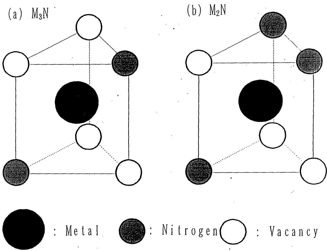
Fig. 9. Two types of environments around a metal site in  $M_3N$  (a) and  $M_2N$  (b).
