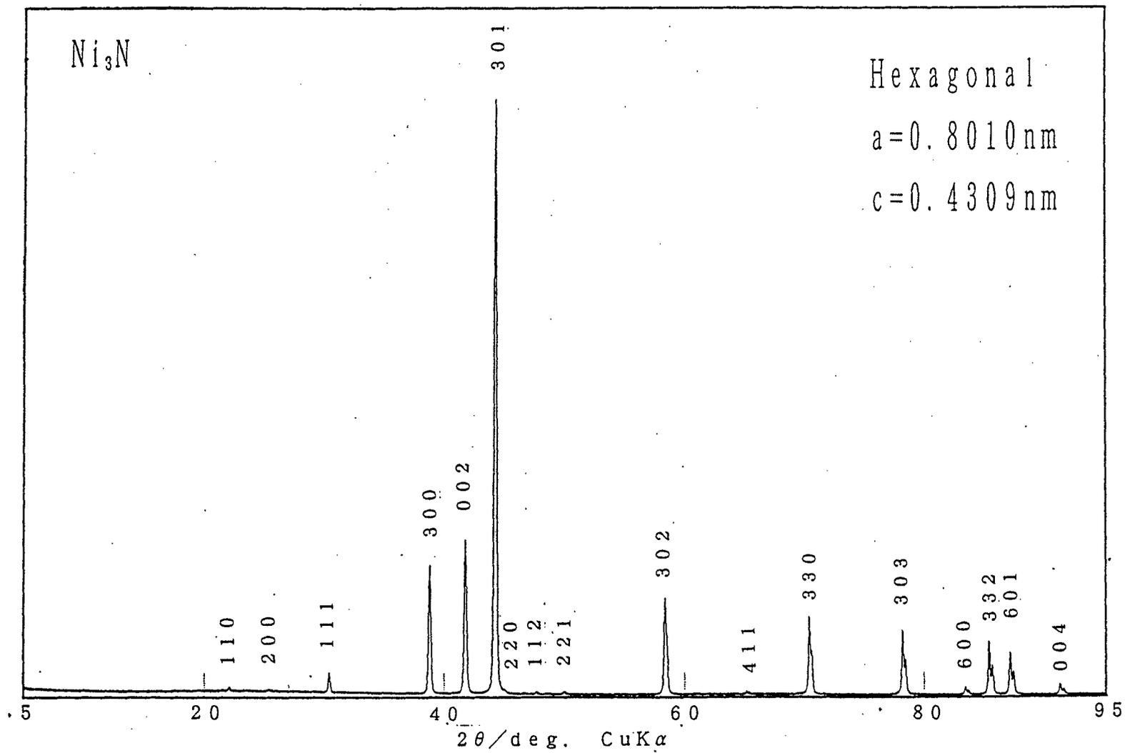
Fig. 3. X-ray diffraction pattern of  $\text{Ni}_3\text{N}$ .
