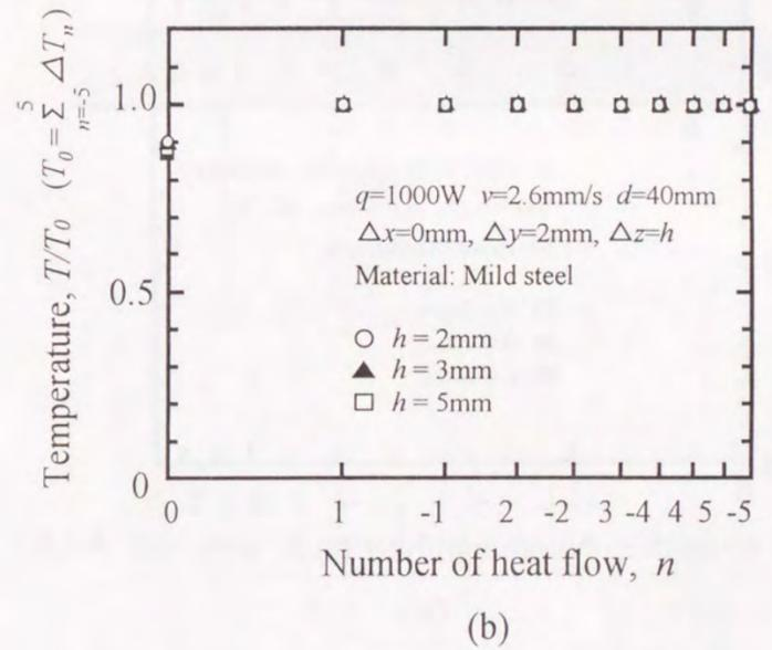
Fig.5-2 Influence of total number of heat flow in circumferential direction on temperature field in arc welding on mild steel pipe ( $n>0$ :clockwise direction,  $n<0$ :anticlockwise direction) (a)  $d=20\text{mm}$  (b)  $d=40\text{mm}$
