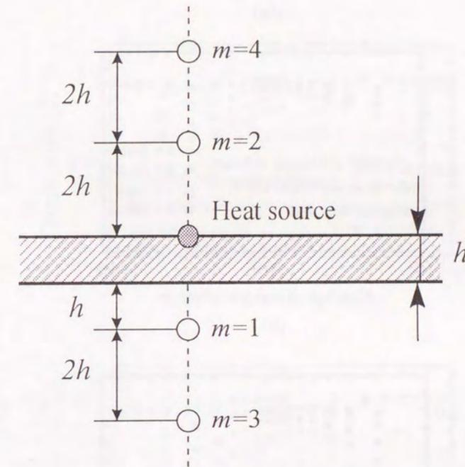
Fig.5-4 Schematic of imaged heat source in welding on thin plate
