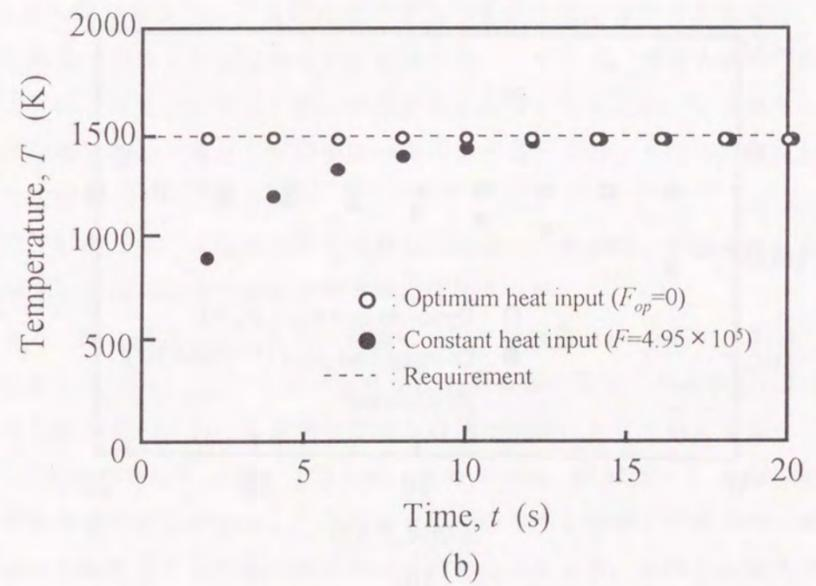
Fig.2-6 Comparison of temperature at target point calculated by optimum heat input and constant one (Material:Mild steel)
