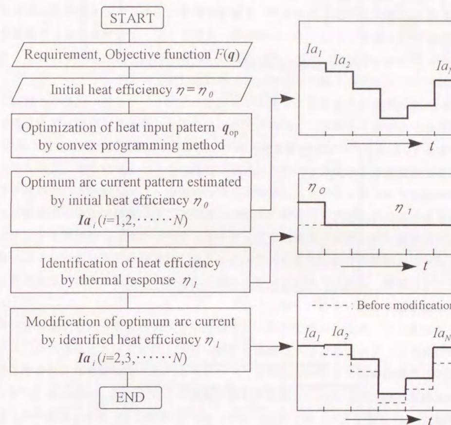
Fig. 4-15 Flow chart of in-process identification of model parameter  $\eta$
