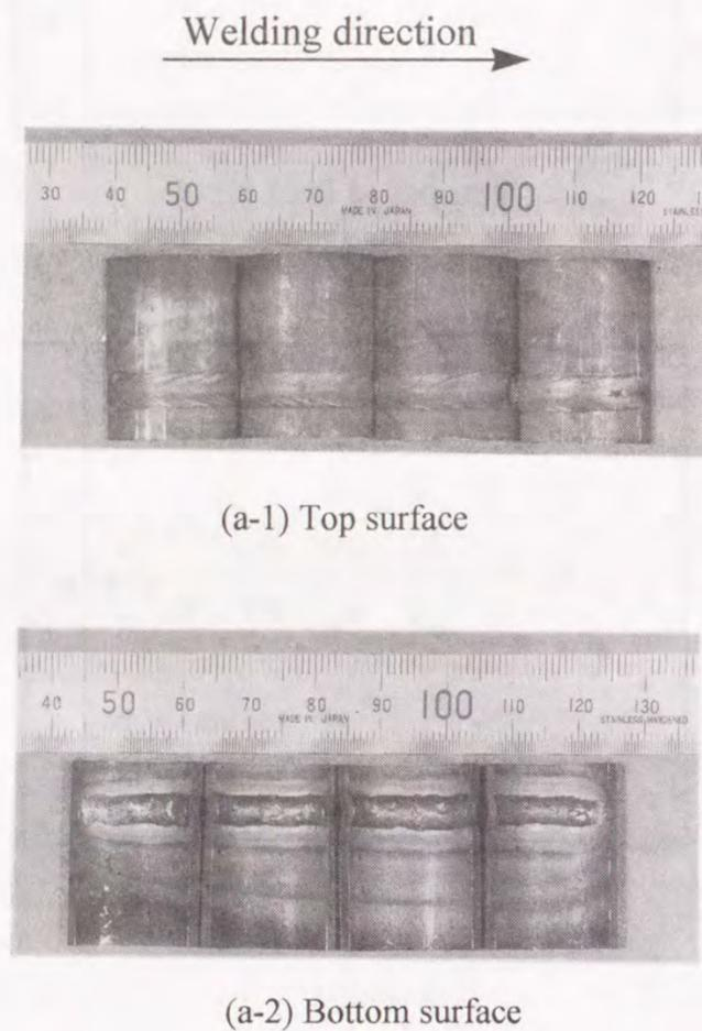
Fig.5-14 Appearance of top and bottom surface after welding on mild steel pipe
