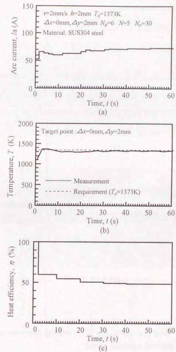
Fig.6-8 Modified optimum arc current and temperature at target point in process of real-time optimum control ( $L_{a_s}=2\text{mm}$ ,  $L_{a_f}=12\text{mm}$ )
