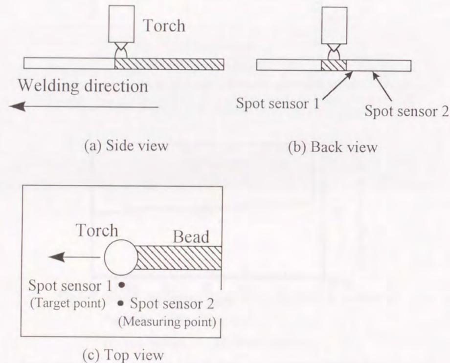
Fig.6-11 Schematic of measuring method for temperature at bottom surface by spot sensor in GTA welding on thin plate
