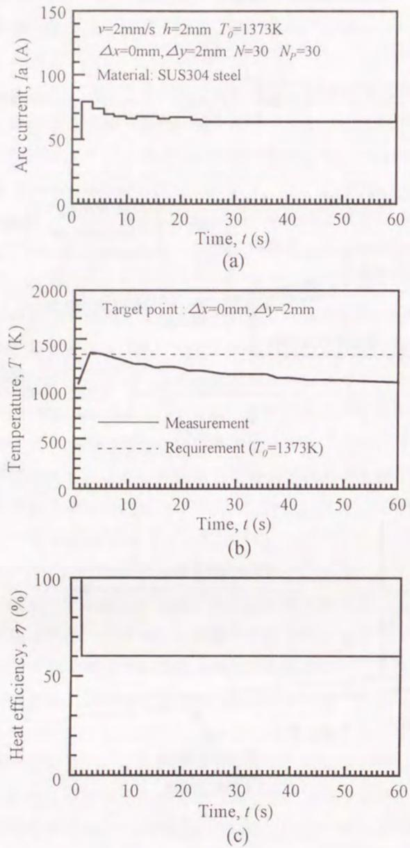
Fig.6-6 Influence of change in arc length on temperature field in GTA welding on SUS304 steel plate ( $L_{a_s}=2\text{mm}$ ,  $L_{a_f}=12\text{mm}$ )
