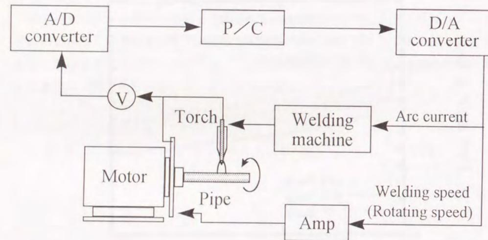
Fig.5-12 Schematic of GTA welding apparatus on rotating pipe
