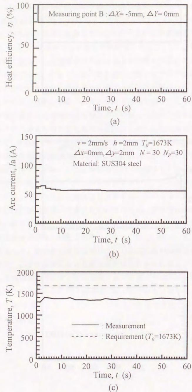
Fig.4-17 In-process identification with use of thermal response at measuring point B
