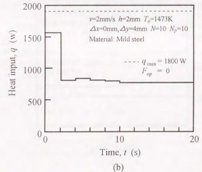
Fig.3-8 Comparison of optimum heat input pattern estimated by steepest descent method and convex programming method (Without active constraint)
