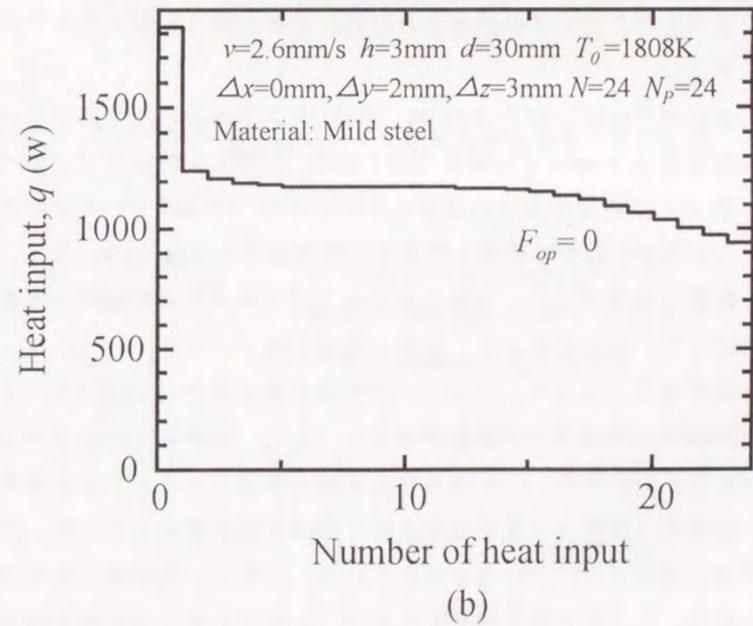
Fig.5-7 Comparison of optimum heat input pattern for welding on between thin mild steel plate and mild steel pipe
