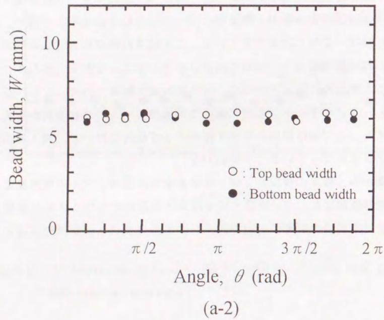
Fig.5-16 Comparison of bead width in welding on aluminum pipe with between optimum heat input and constant one
