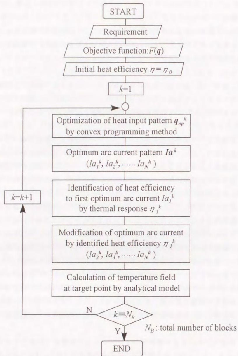
Fig.6-1 Flow chart of real-time optimization algorithm of heat input pattern by convex programming method with use of in-process identification of heat efficiency by thermal response
