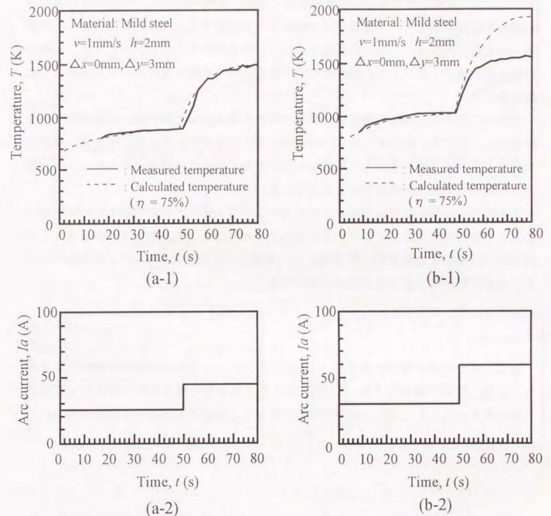
Fig.4-13 Comparison between measured and calculated thermal response in GTA welding on mild steel plate
