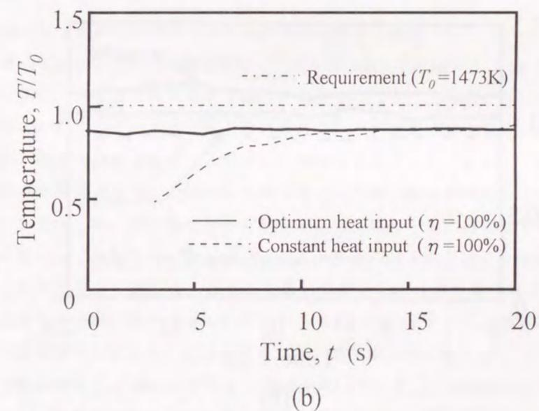
Fig.4-3 Experimental result of optimum heat input estimated by convex programming method compared with constant one
