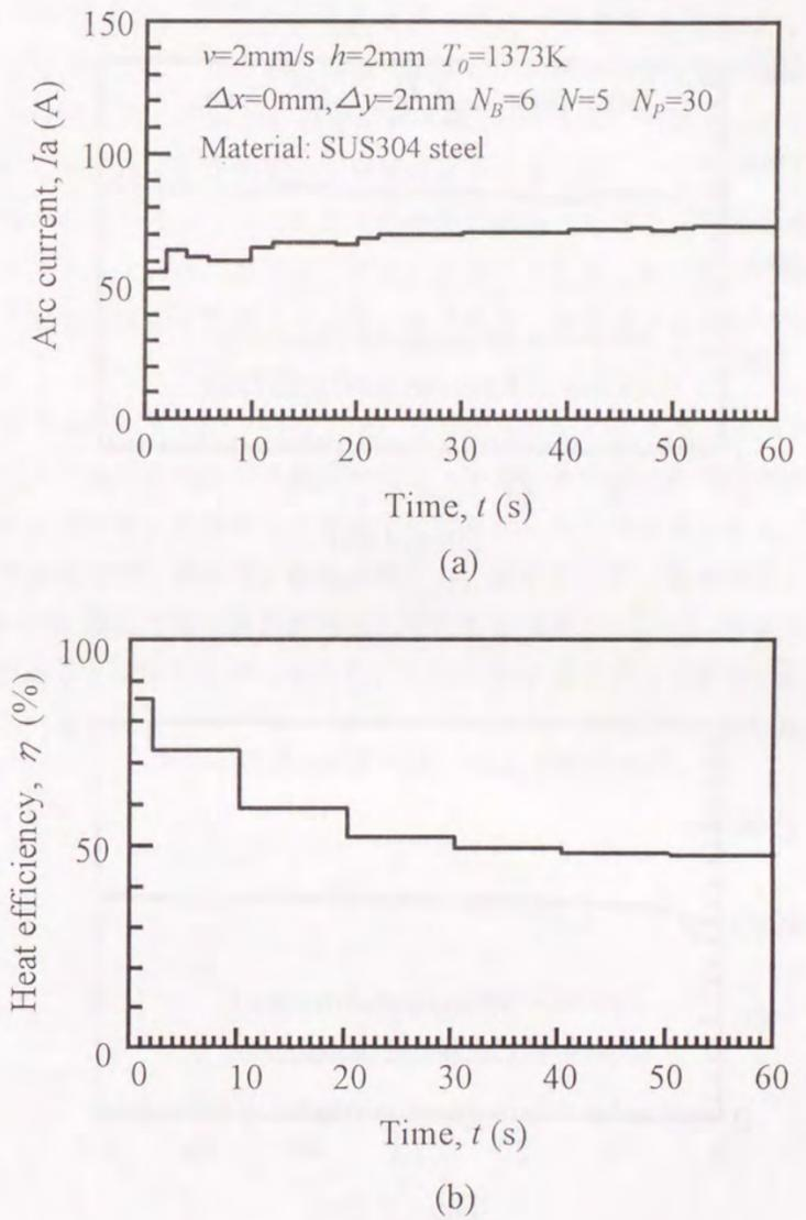
Fig.6-14 Controlled temperature in process of real-time identification of heat efficiency by thermal response ( $L_{a_s}=2\text{mm}$ ,  $L_{a_f}=12\text{mm}$ )
