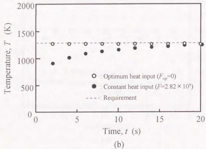
Fig.2-7 Comparison of temperature at target point calculated by optimum heat input and constant one (Material:Copper)
