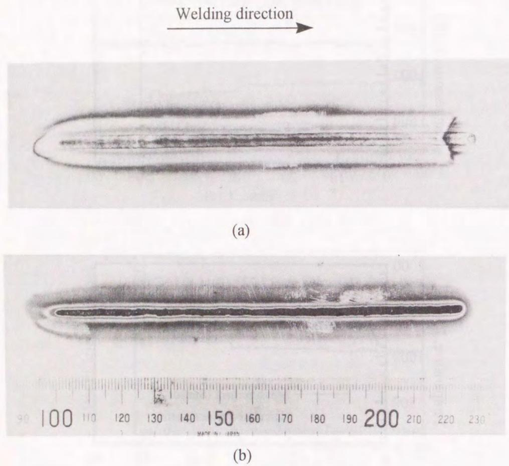
Fig.6-13 Bead appearance after GTA welding in-process of real-time optimum control
