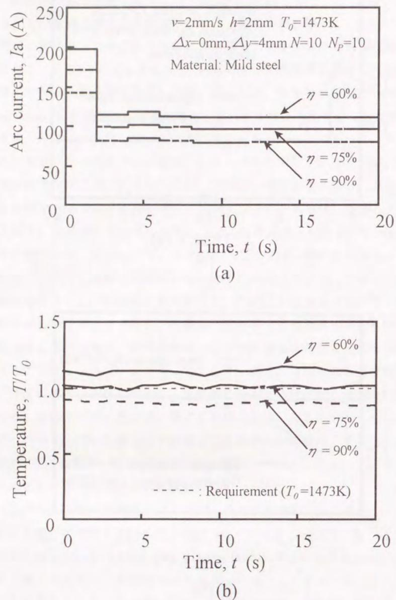
Fig.4-4 Influence of heat efficiency on temperature field in welding with optimum heat input
