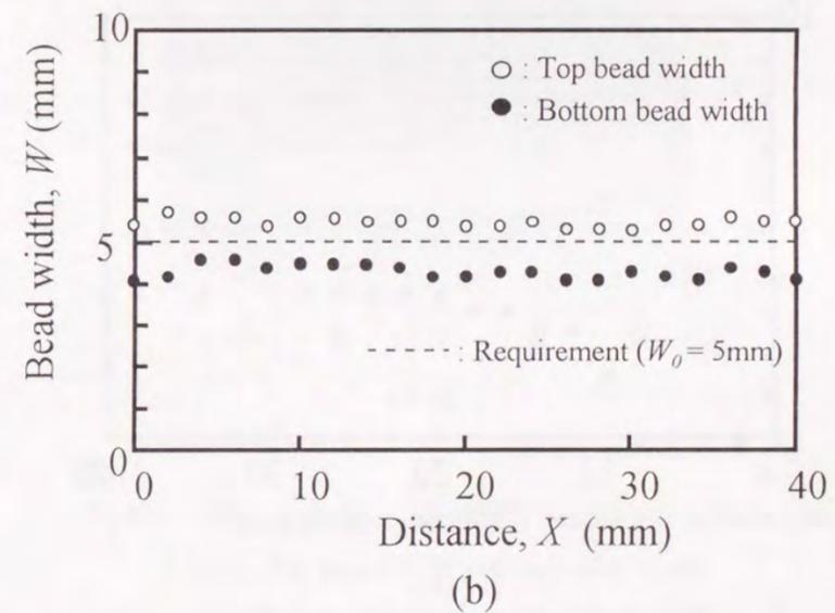
Fig.4-8 Experimental result of heat input optimized by steepest descent method
