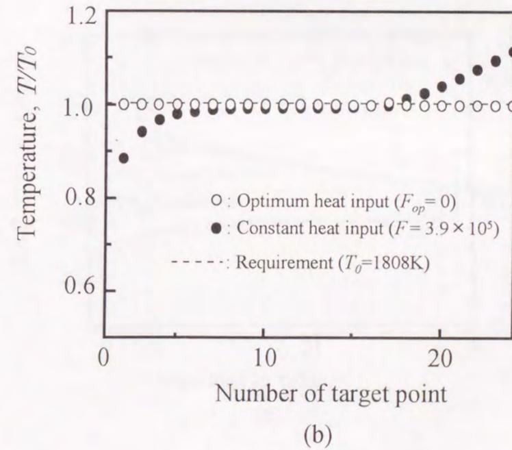
Fig.5-8 Calculated temperature field in arc welding on mild steel pipe by using optimum heat input and constant one
