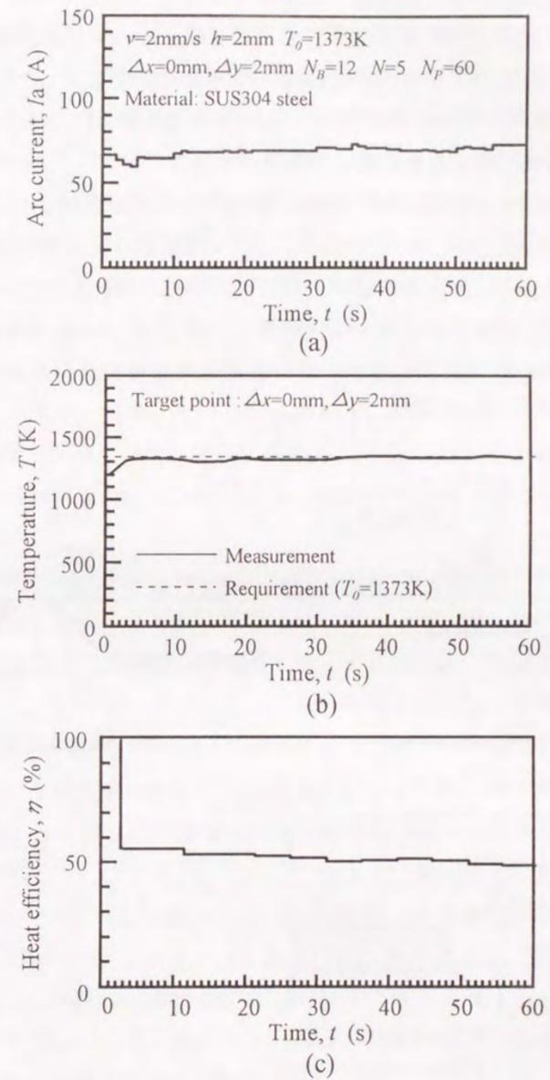
Fig.6-10 Modified optimum arc current and temperature at target point in process of real-time optimum control ( $L_{a_s}=2\text{mm}$ ,  $L_{a_f}=12\text{mm}$ )
