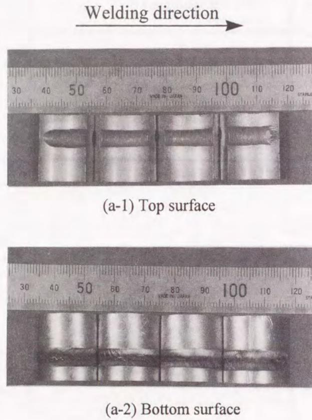
Fig.5-17 Appearance of top and bottom surface after welding on aluminum pipe
