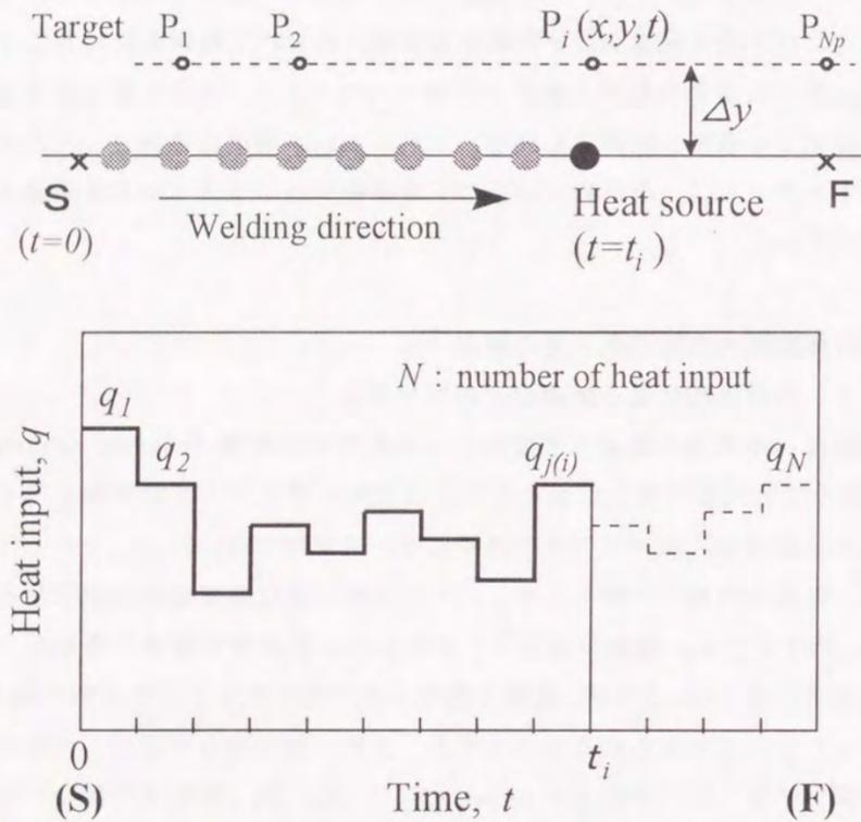
Fig.2-1 Typical example of convex programming problem in arc welding
