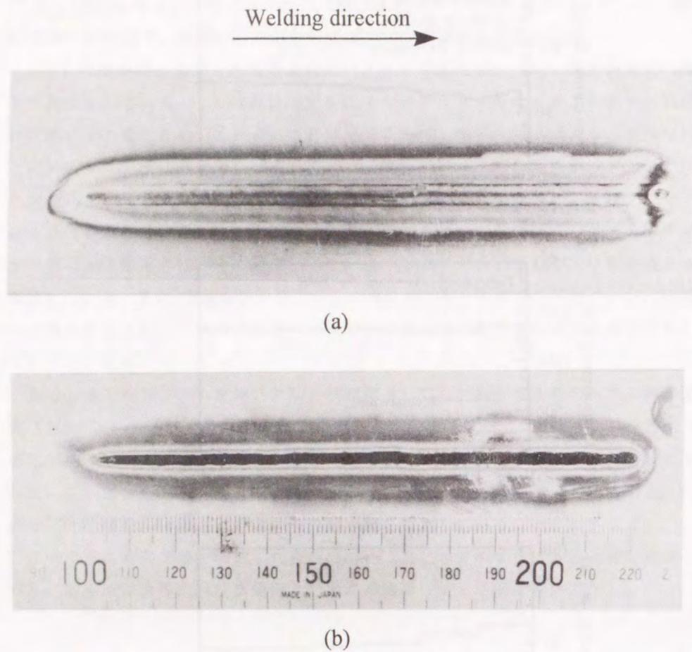
Fig.6-9 Bead appearance after GTA welding in-process of real-time optimum control
