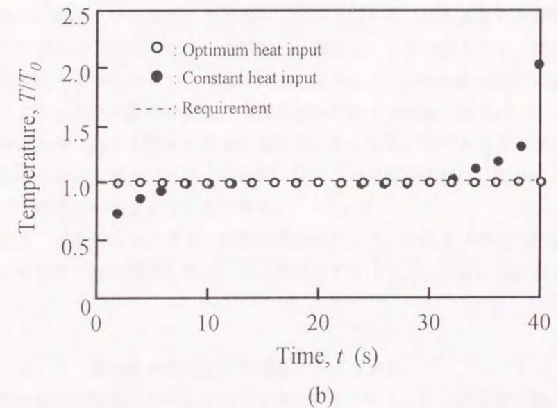
Fig.2-9 Calculation result of optimum heat input in arc welding on thin plate with finite length
