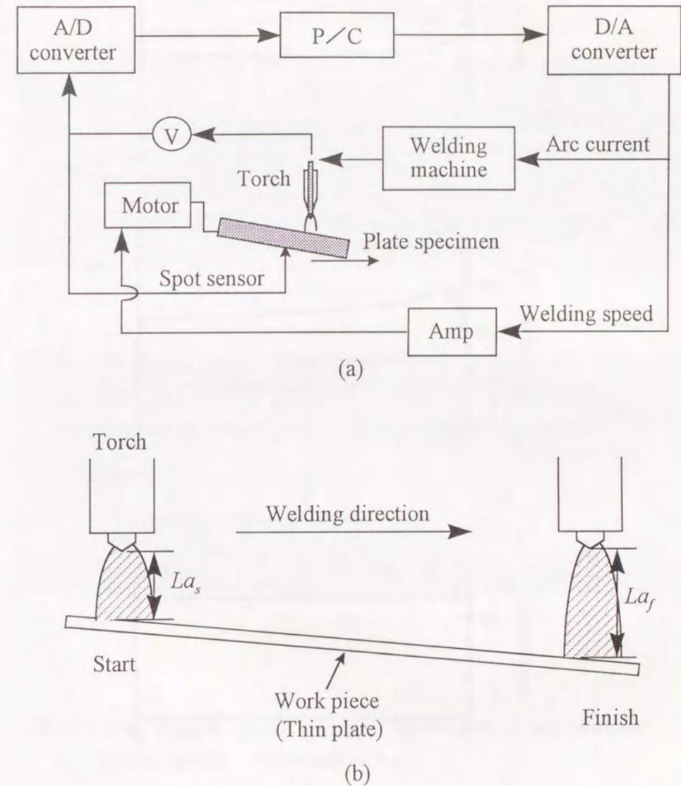
Fig.6-5 Schematic of experimental procedure with change in arc length during GTA welding on thin plate
