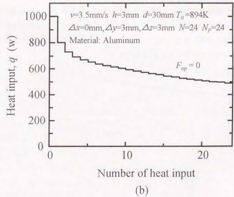
Fig.5-10 Influence of total number of heat input on optimum heat input pattern in arc welding on aluminum pipe
