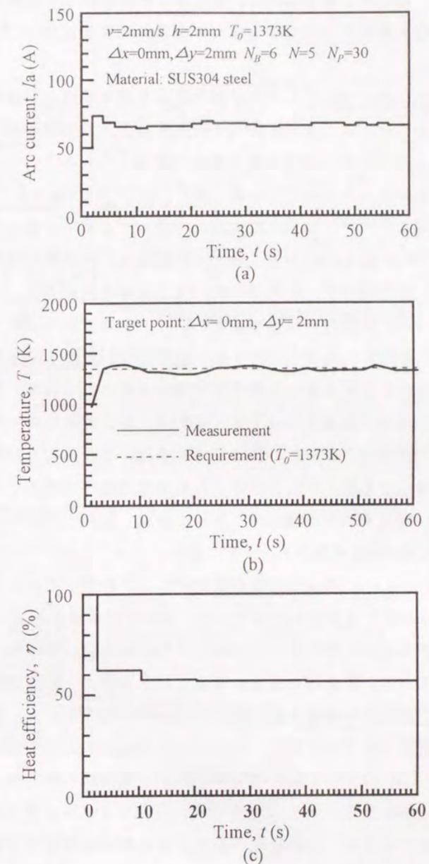
Fig.6-4 In-process identification of heat efficiency in GTA welding on SUS304 steel plate ( $L_a=2\text{mm}$ ,  $L_f=2\text{mm}$ )
