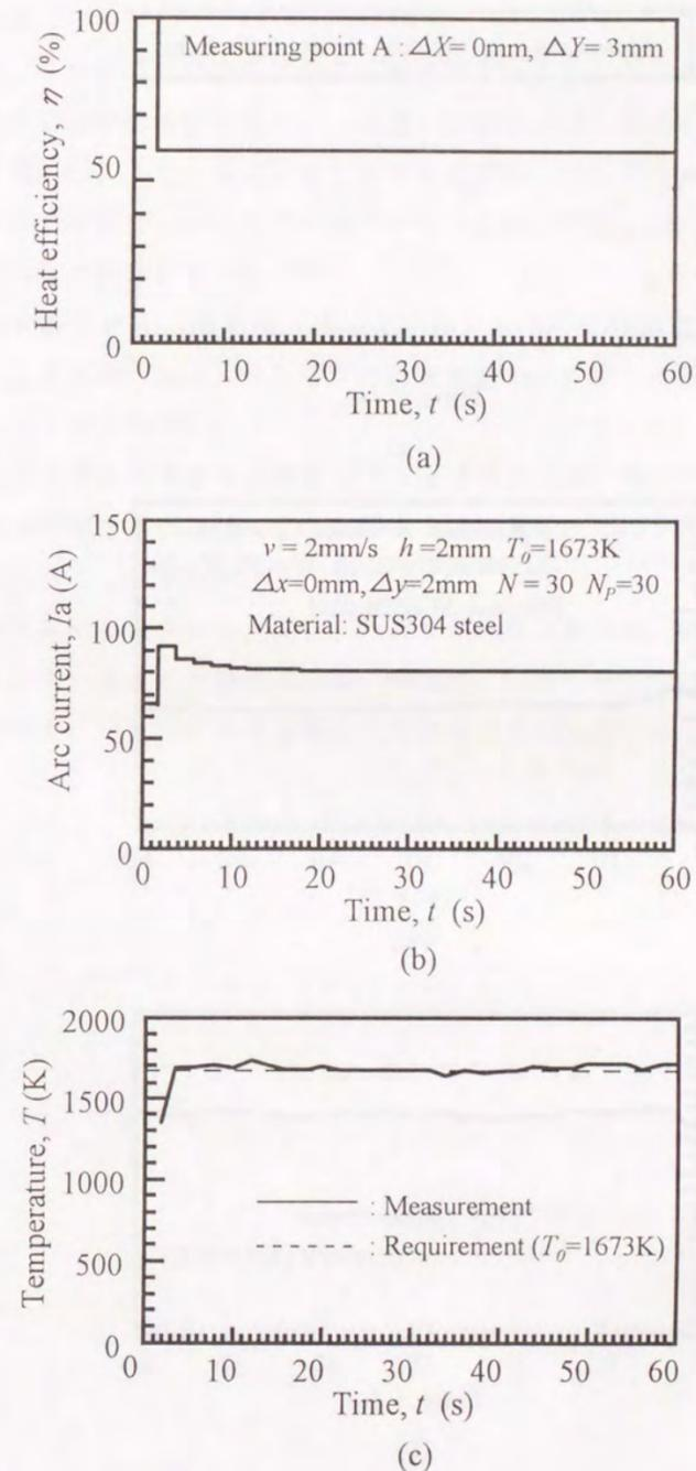
Fig.4-16 In-process identification with use of thermal response at measuring point A
