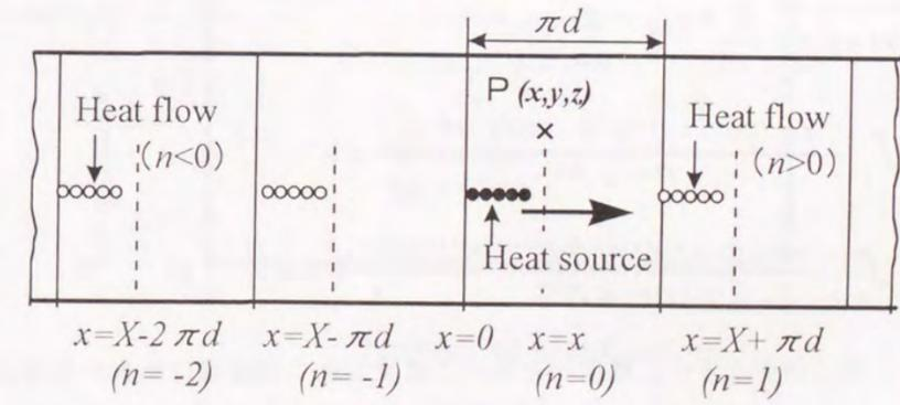
Fig.5-1 Schematic of arc welding on pipe and heat flow in circumferential direction during welding ( $n<0$ :clockwise direction,  $n>0$ :anticlockwise direction)
