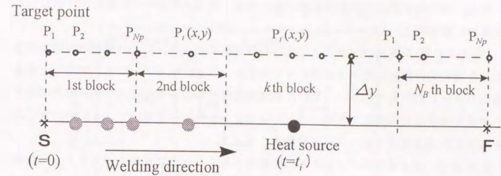
Fig.6-2 Real-time optimization problem of temperature field in GTA welding
