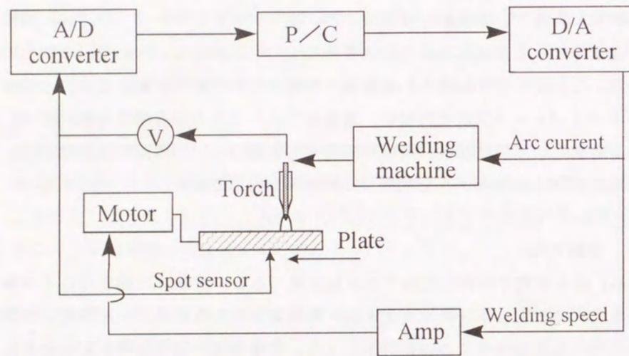
Fig.4-1 Schematic of experimental apparatus of GTA welding
