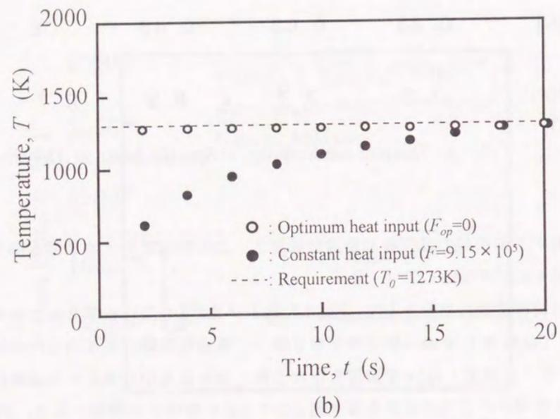
Fig.2-5 Comparison of temperature at target point calculated by optimum heat input and constant one (Material:Mild steel)
