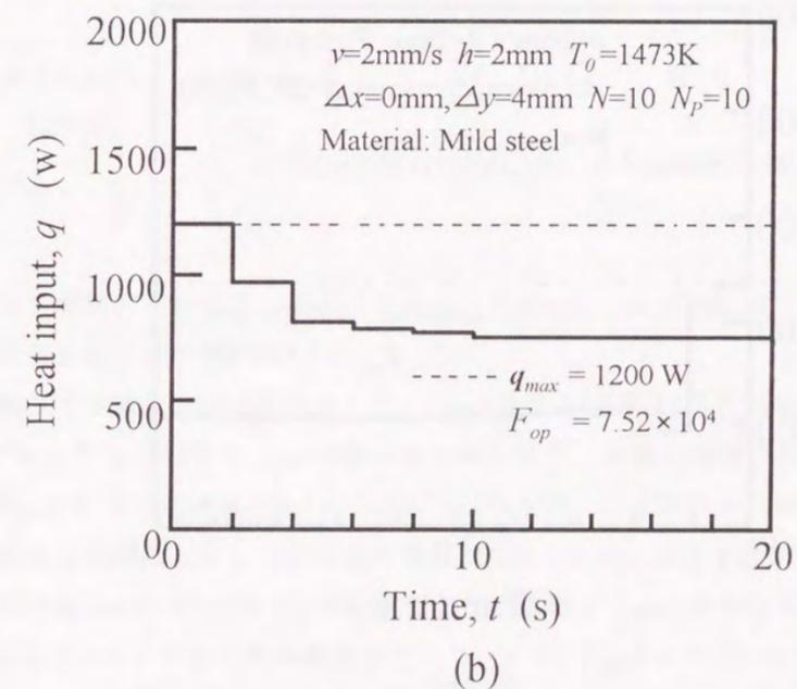
Fig.2-3 Calculated result of optimum heat input in welding on mild steel plate
