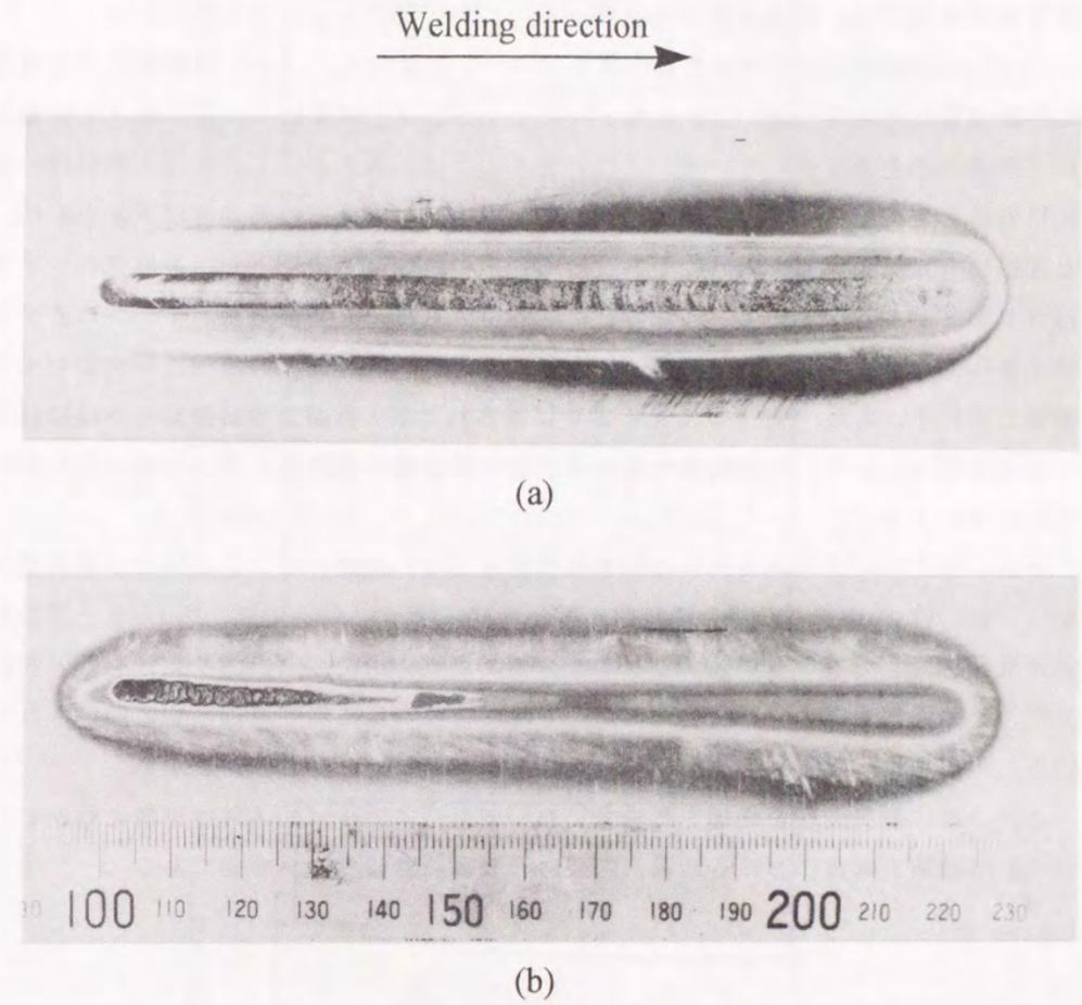
Fig.6-7 Bead appearance under in-process identification of heat efficiency
