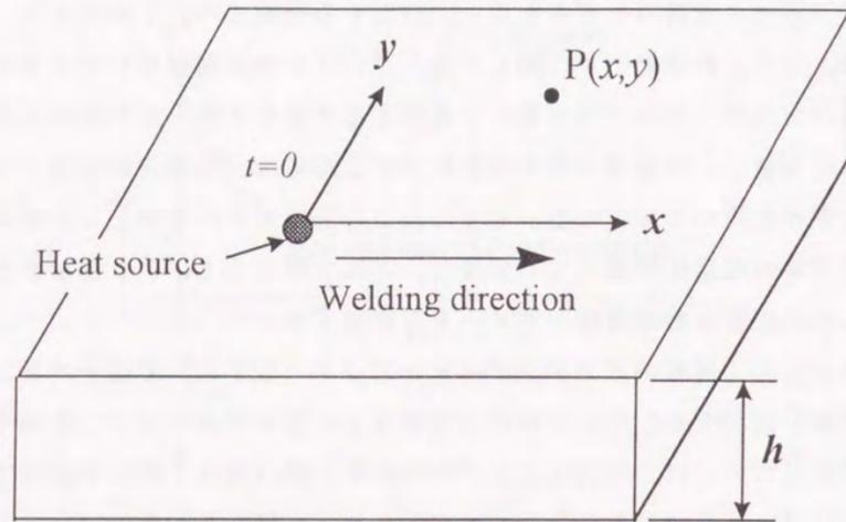
Fig.1-2 Model of moving heat source in arc welding on infinite plate
