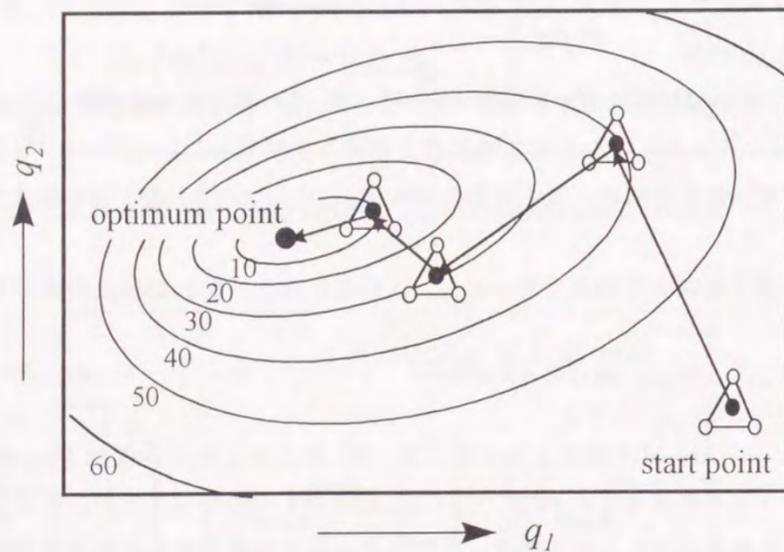
Fig.3-2 Schematic in process of searching by steepest descent method (2 factors)
