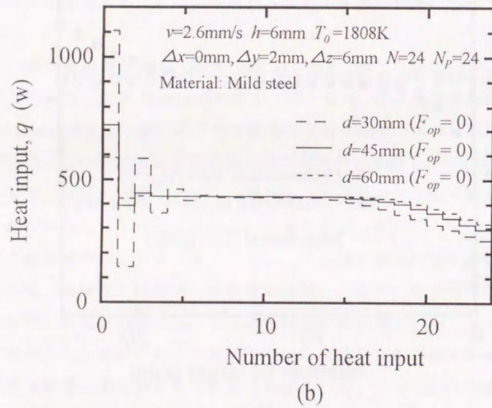
Fig.5-9 Influence of thickness and diameter of pipe on optimum heat input pattern in arc welding on mild steel pipe
