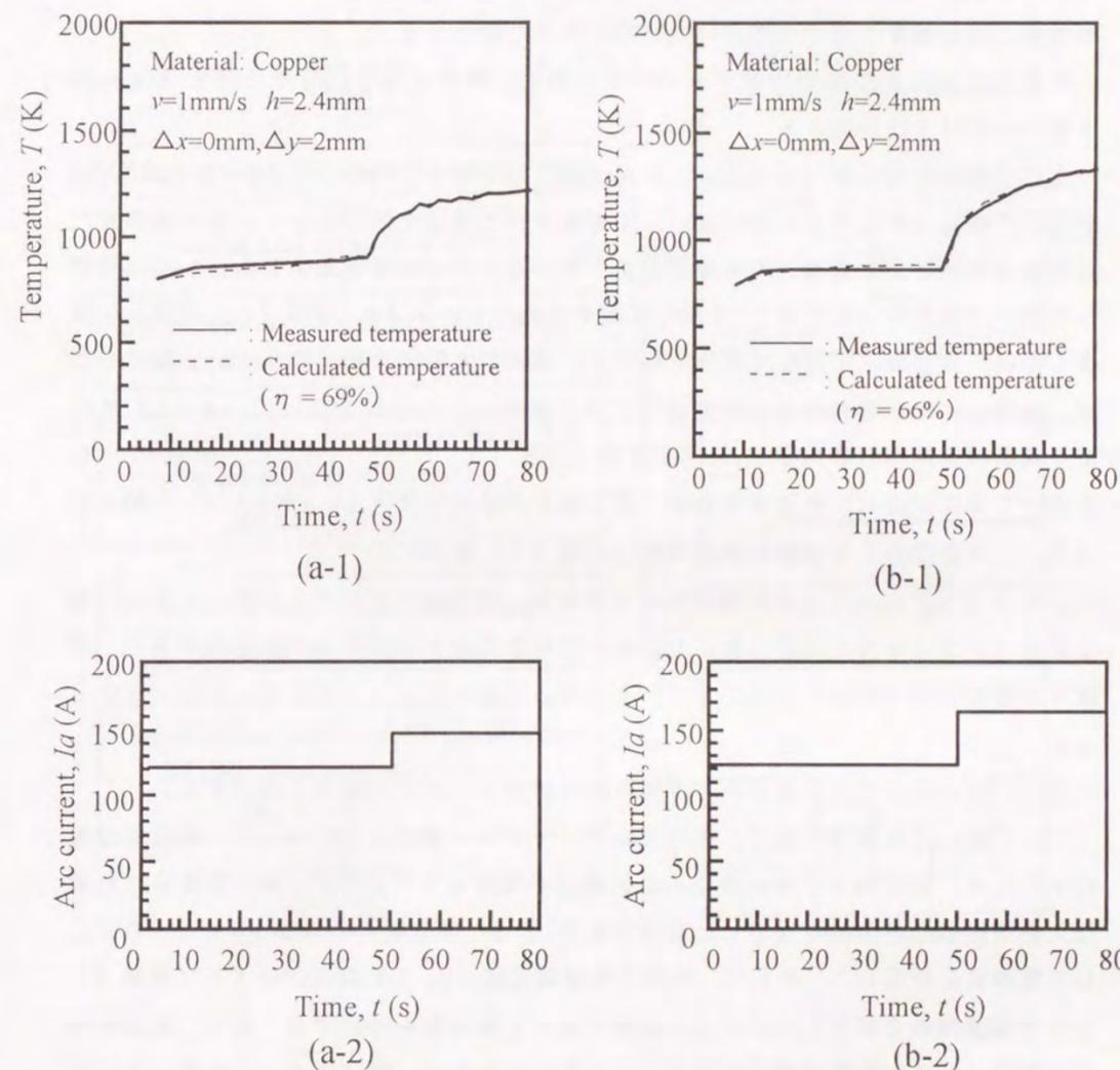
Fig4-14 Comparison between measured and calculated thermal response in GTA welding on copper plate
