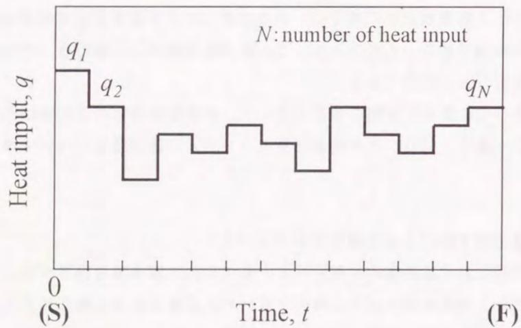
Fig.3-1 Optimization problem to control maximum temperature in arc welding on plate specimen
