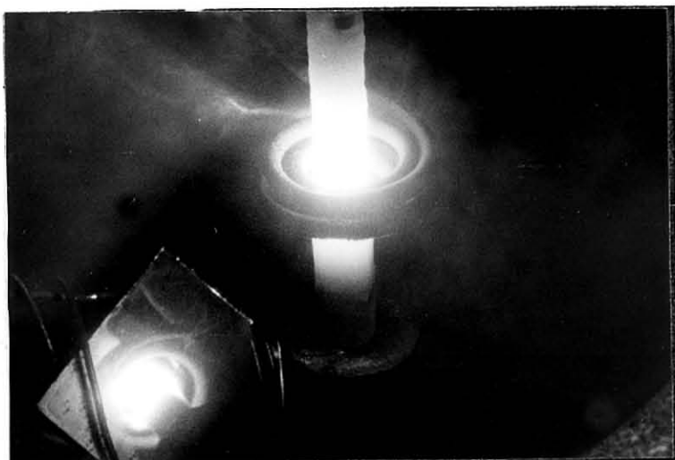
Fig.2-12. Floating zone experiment observed through view port.
