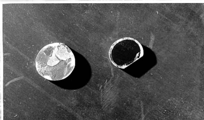
Fig.2-21. Photograph of the as-grown ZrB_2 crystal whose surface has golden luster due to ZrN formation.
