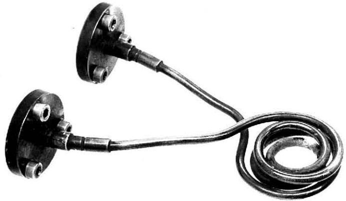
Fig.2-8. Work coil for floating zone method. It is made by water cooled copper pipe of 3 mm outer diameter.
