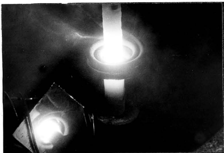
Fig.2-12. Floating zone experiment observed through view port.
