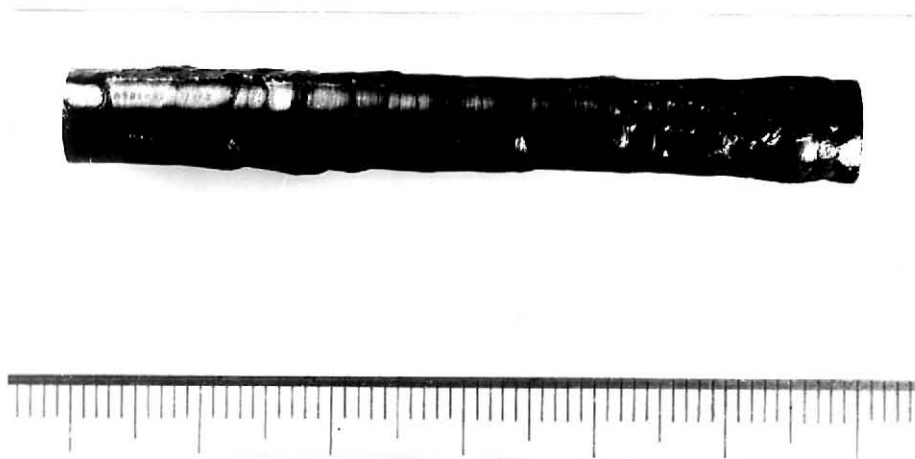
Fig.2-13. Photograph of the as-grown \text{LaB}_6 crystal.
