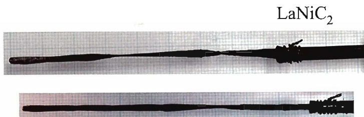
Fig. 4.14 Single crystal ingots of \text{LaNiC}_2 grown by the Czochralski method.
