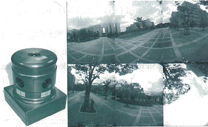
Fig 1.4 Omni-directional multi-camera system for positioning [1-17]
