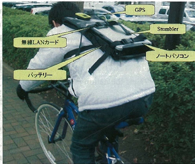
Fig 5.2 Locating the Wi-Fi access points[5-2]
