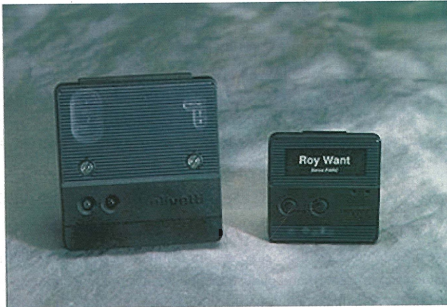
Fig 2.6 Olivetti Active Badge (right) and a base station (left)
