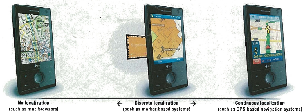
Fig 3.3 Marker-based positioning and continuous positioning
