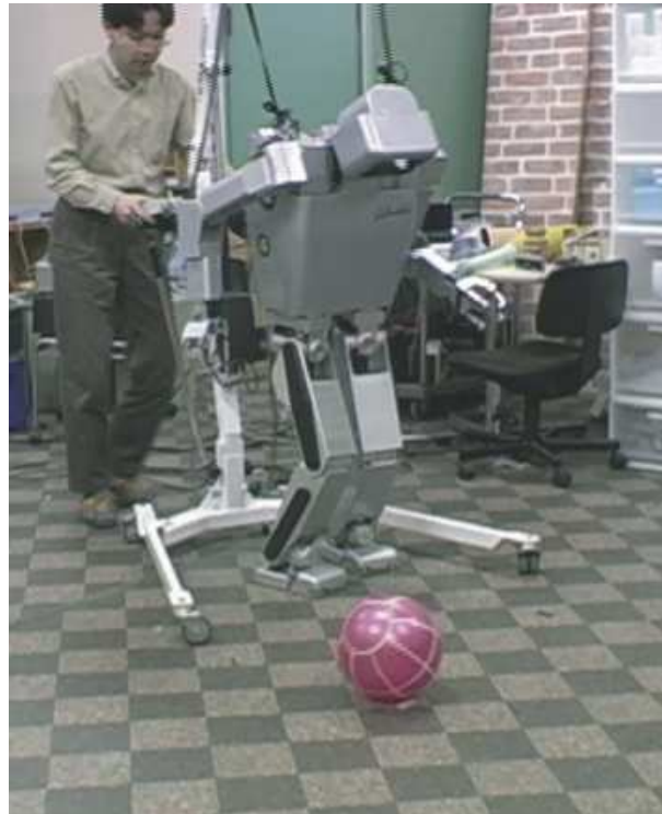
FIGURE 5.2: A humanoid robot can chase a moving ball by predicting its motion.: from [82]
