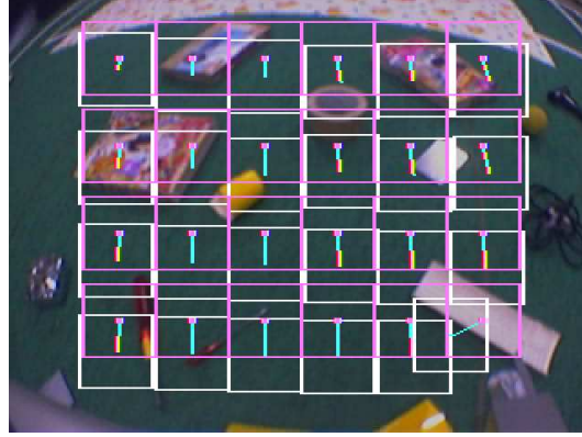
FIGURE 7.5: An example of an optic flow in the robot's view
