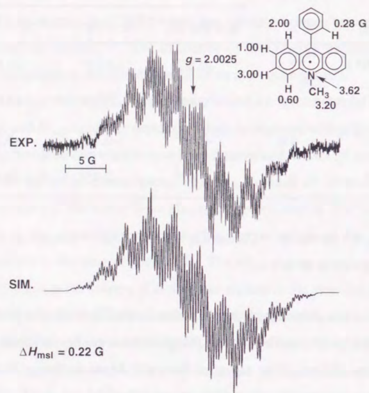
Figure 2. ESR spectrum of MeAcrPh • in deaerated MeCN at 298 K and the computer simulation spectrum.
