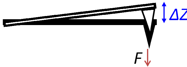
Fig.1.6 Cantilever deflects as the tip is pushed towards the sample
