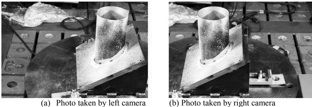
Fig. 1 Photographs of specimen whose angle of joint plane is 30 degree.
