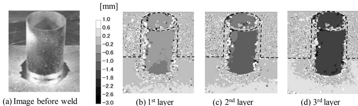
Fig. 2 Distribution of axial displacement measured by 3D measurement based on stereo imaging technique.
