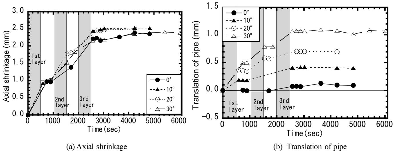
Fig. 3 Influence of inclination angle of joint plane on welding distortion.
