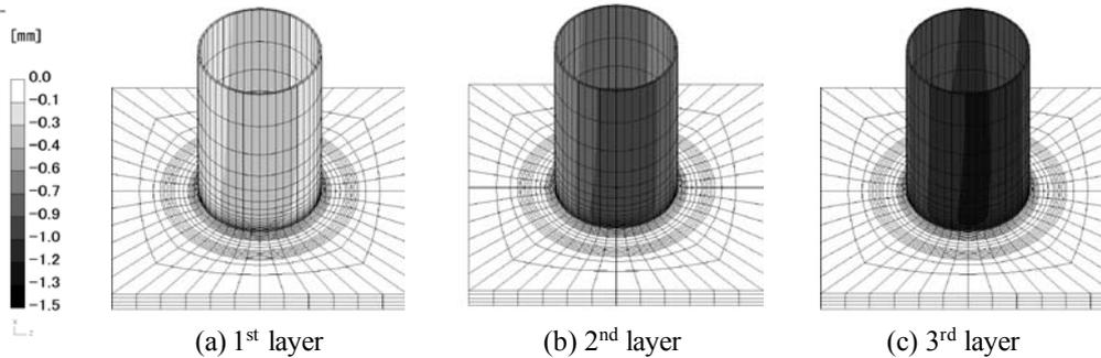
Fig. 4 Distribution of axial shrinkage simulated by Iterative substructure method.
