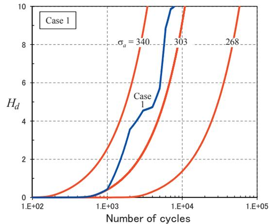
Fig.4 Evolution of plastic strain range and damage parameter  $H_d$  with the increase of number of cycles (Case 1)
