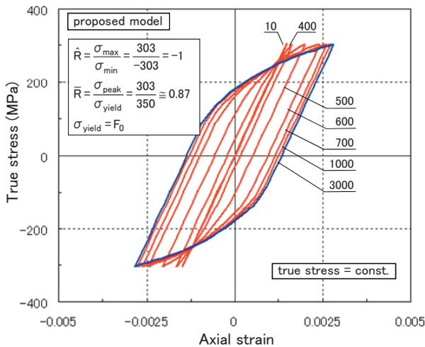
Fig.2 Stress-strain curve under symmetrical cyclic loading
