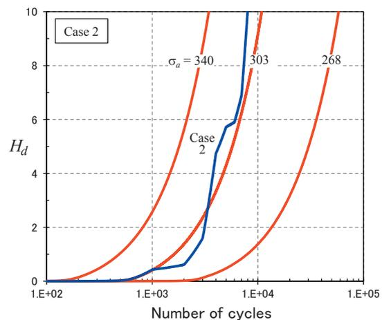
Fig.5 Evolution of plastic strain range and damage parameter  $H_d$  with the increase of number of cycles (Case 2)
