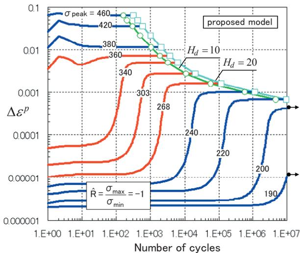
Fig.3 Evolution of plastic strain range with the increase of number of cycles
