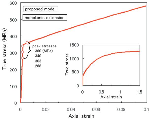
Fig.1 Stress-strain relation predicted by the proposed model under monotonic extension loading
