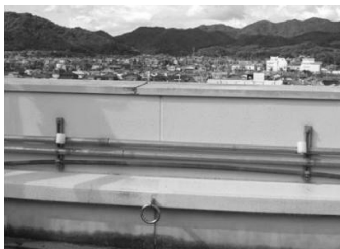
Fig. 5-3 The installation situation of the passive sampler inside rain shelter.
