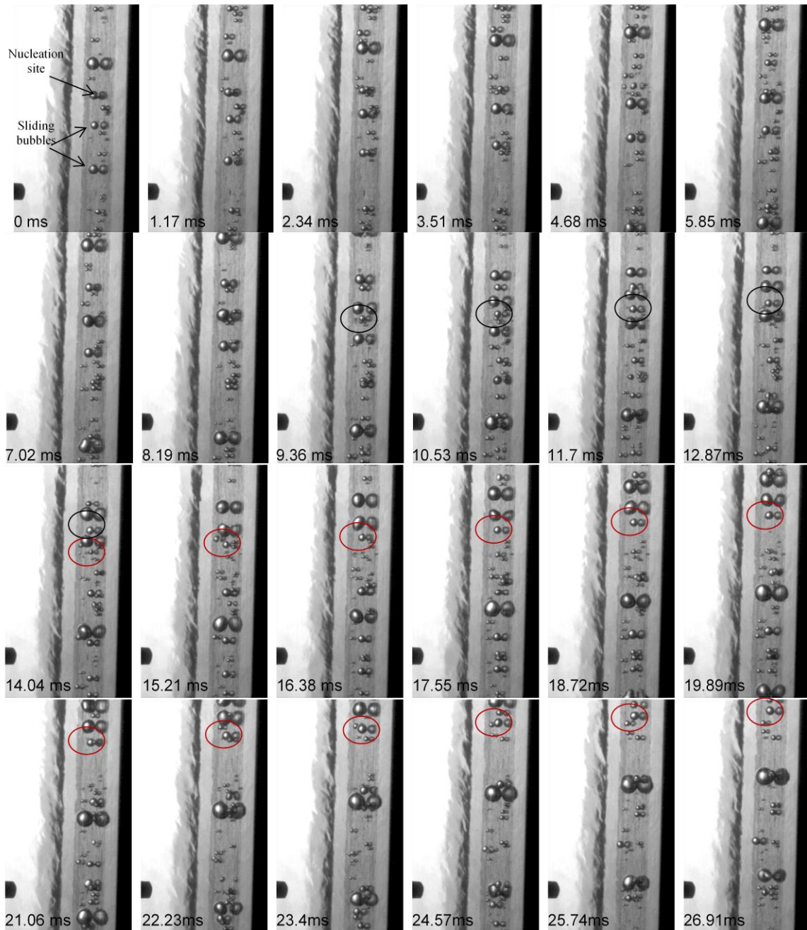
Fig. 6.6 Example of bubble generation in the wake region of preceding sliding bubbles close to OSV condition in Exp. P2.2, Run 2202
