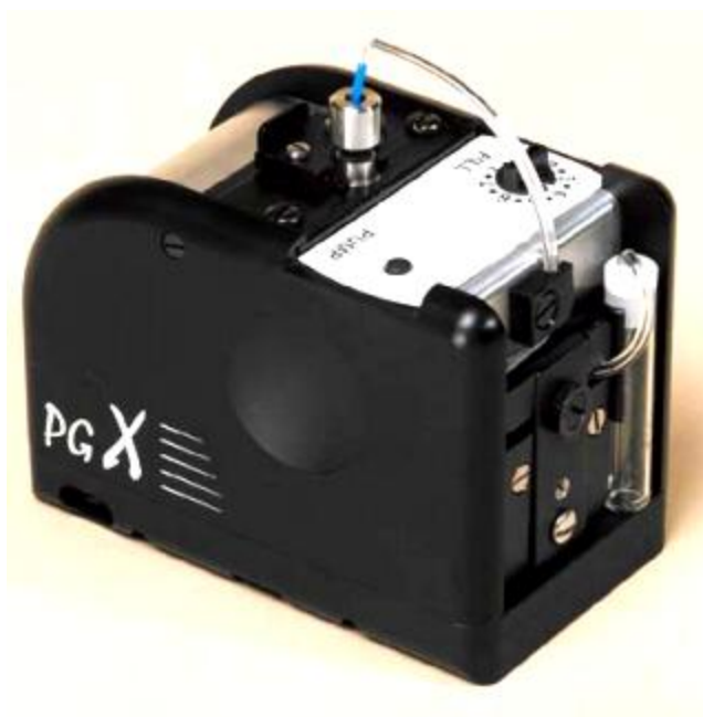
Fig. 2.4 Contact angle measurement instrument PG-X model
