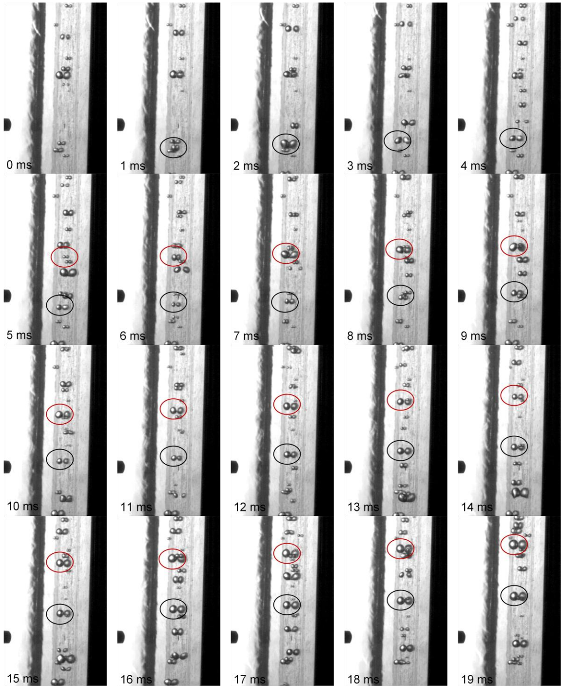
Fig. 6.5 Example of bubble reattachment close to OSV condition in Exp. P1.1, Run 1102
