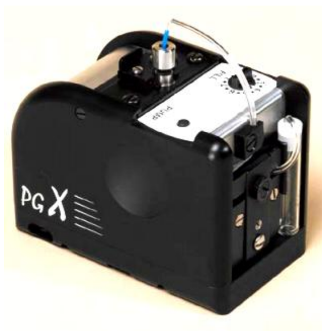
Fig. 2.4 Contact angle measurement instrument PG-X model
