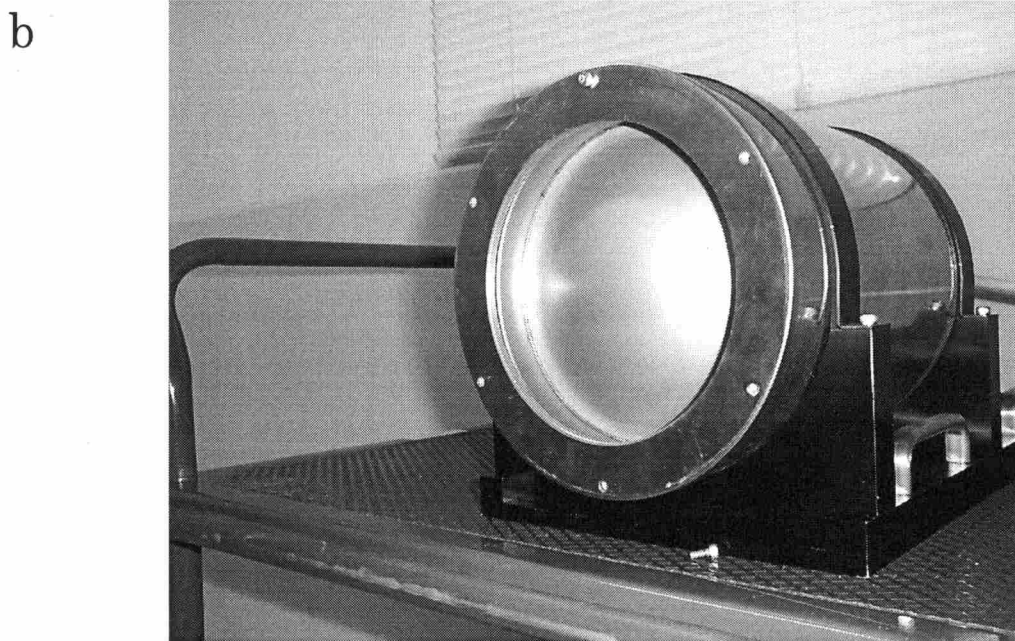
Figure 2.4. (a) Layout of time resolved x-ray diffraction experiments. (b) X-ray image intensifier.
