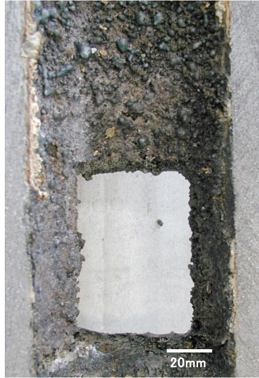
Fig. 6-26. Comparison of internal view of port after 450ton casting (Wakayama)
