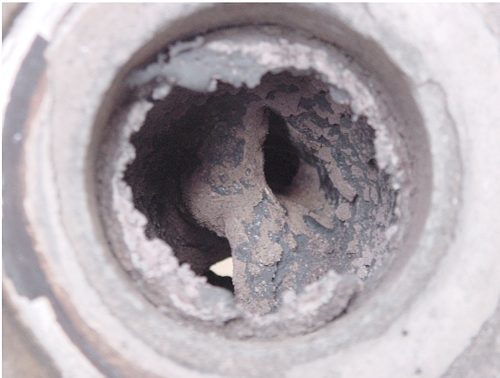
Fig. 6-24. Top view of swirl blade in nozzle after 450ton casting (Wakayama).
