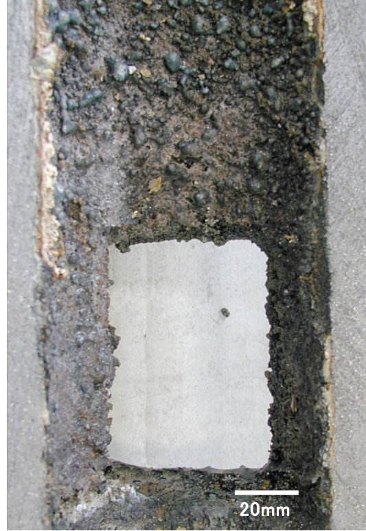
Fig. 6-26. Comparison of internal view of port after 450ton casting (Wakayama)
