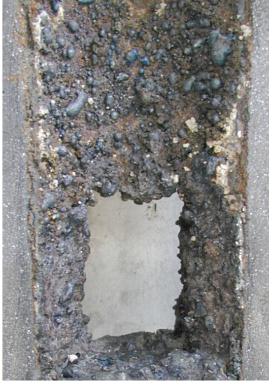
Fig. 6-26. Comparison of internal view of port after 450ton casting (Wakayama)
