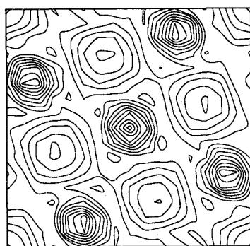
Fig. 6.3.8 Valence electron density on  $z = 0$  plane (grain boundary plane) for  $\Sigma = 5[001]$  twist grain boundary for the atomic structure calculated by EMT which is used as the initial state for FP-MD. The interval of contour is  $2.5 \times 10^{-3}$  in atomic unit.
