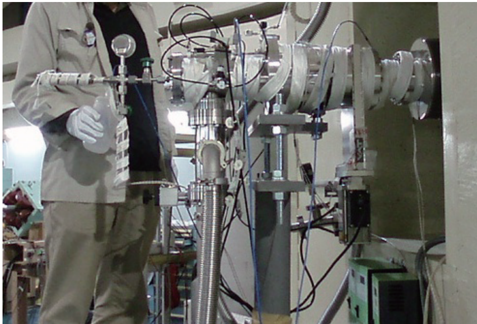
Figure 4.2: The view of the experimental port during the baking. The white belts are the ribbon heaters. The apparatus attached to the experimental port is used for the deuteration.
