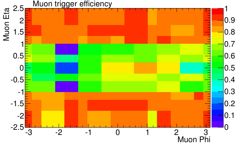
Figure 5.5: The muon trigger efficiency measured in data in the \eta - \phi plane. The low efficiency region at \phi \sim -1.8 is due to the ATLAS support structure.
