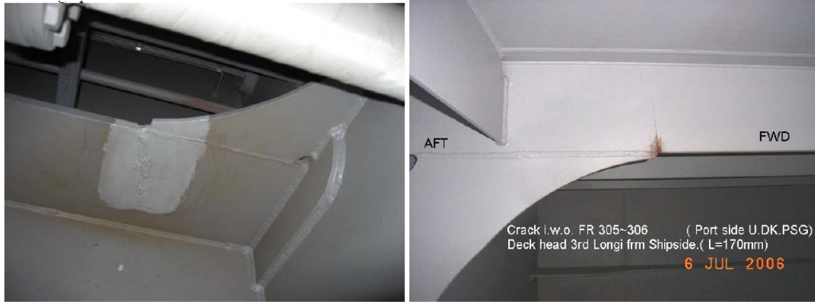
(a) a crack on upper inner side longitudinal (b) a crack in deck longitudinal
