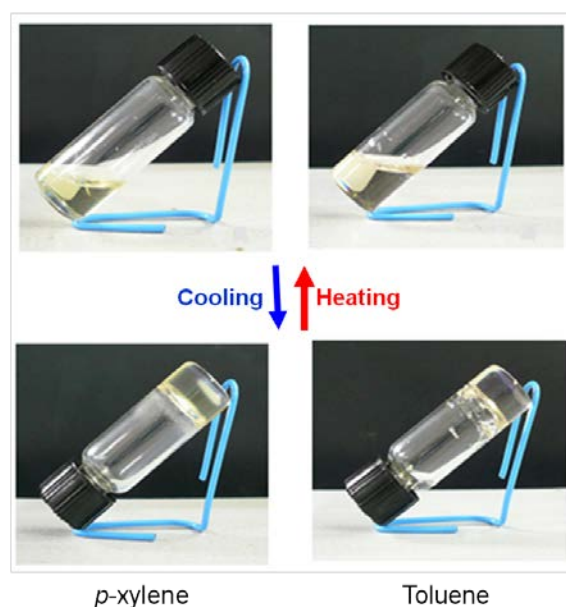
Figure 5-4. Real images of the reversible transition of gel-solution states in p -xylene and toluene.
