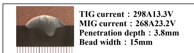
Fig.3.10 Experimental results of penetration shape
