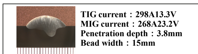
Fig.3.10 Experimental results of penetration shape
