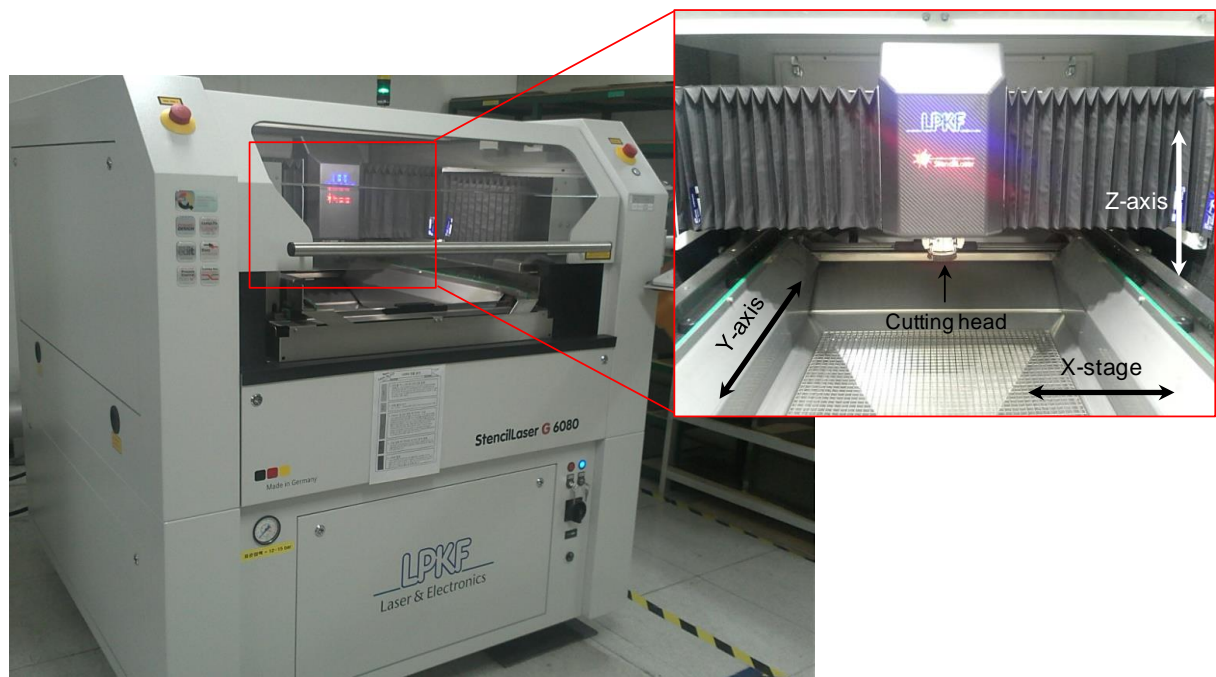
FIGURE 6.4 Photographs of laser-cut system used.
