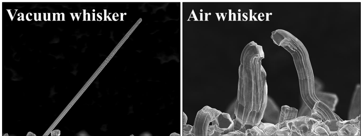
Thermal cycling whisker in vacuum and air (Jung-Lae Jo, 2013)
