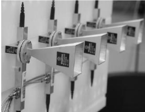
Figure 1-6 (a) Schematic of a converter from wireless microwave to lightwave signals. (b) Examples of antennas combined with EO modulators [30] [37].
