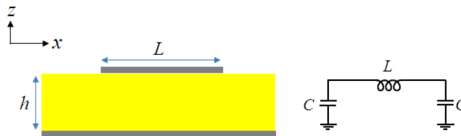
Figure 3-5 Equivalent circuit for the standard patch antenna with no gap.
