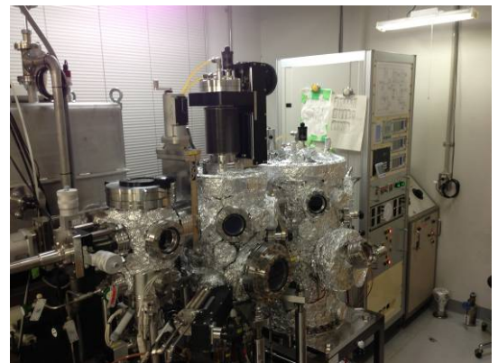
Figure 2-13. A picture of ODA-8300 system. Py, Pd, Al can be evaporated in this
