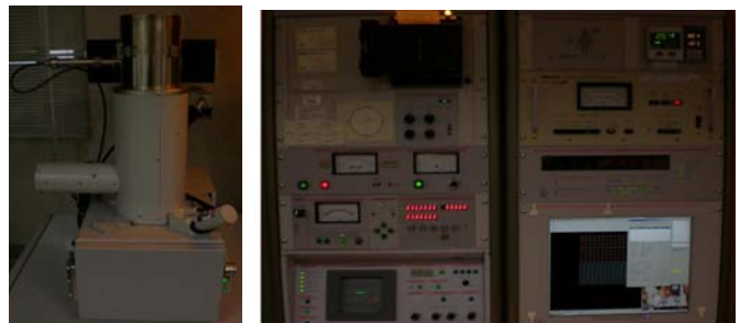
Figure 2-11. The EB lithography system. Sample room (left) and the control unit (right).
