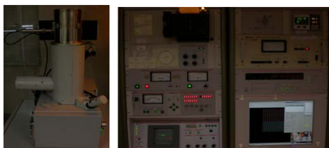
Figure 2-11. The EB lithography system. Sample room (left) and the control unit (right).
