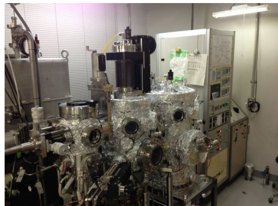
Figure 2-13. A picture of ODA-8300 system. Py, Pd, Al can be evaporated in this system.
