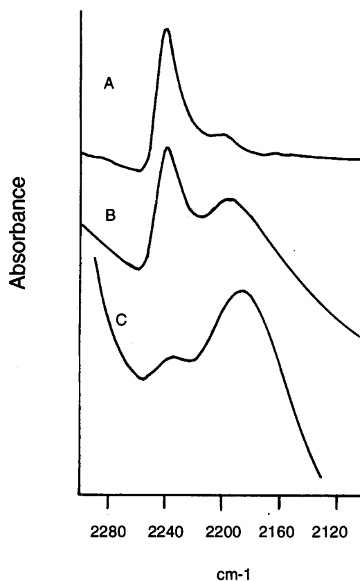
Fig. 7 Change in the absorption intensities of the 2240- and 2190- \text{cm}^{-1} bands the 1 a crystals upon heating at 100^{\circ}\text{C} : the heating times are A, 0 h; B, 25 h; and C, 72 h.
