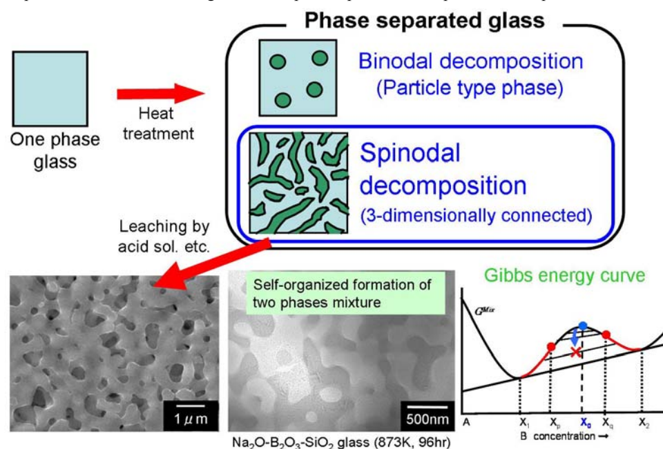
Figure 2 Concept of formation of porous glass materials from spinodal decomposition
