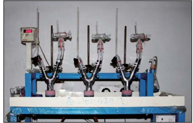
Fig. 20 Mercury apparatus used for H_D measurement
