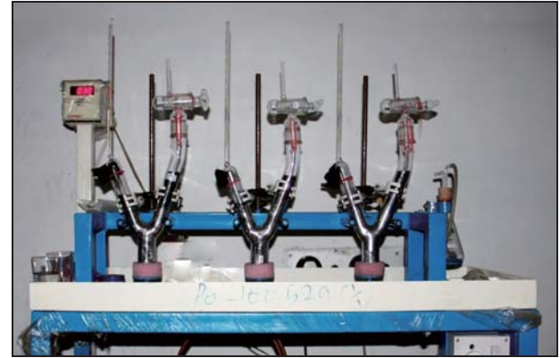
Fig. 20 Mercury apparatus used for H_D measurement
