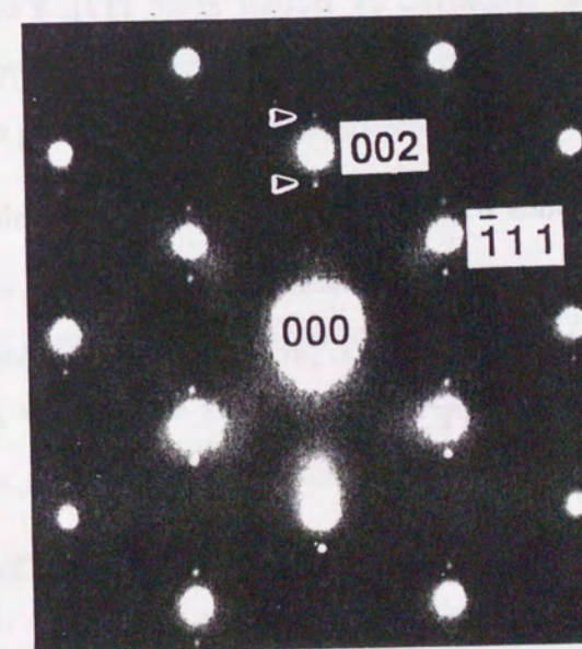
Figure 2-8. A TED pattern from (110) cross-section of (InAs) 4 (InP) 1 sample.
