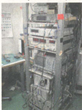
(a) Conventional NMR polarimeter system
