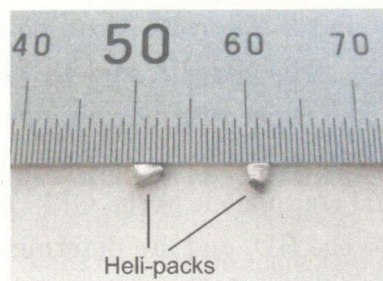
Figure 7.4: Photograph of Heli-packs which are filled into the rectification and reboiler parts.
