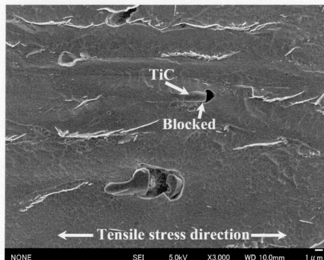
Figure 5.9 Microstructure of high temperature tensile tested sample at necking area revealed retardation of grain boundary sliding by TiC particle.
