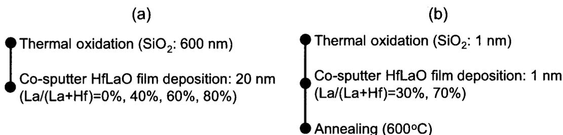
図5.15 HfLaO膜作製フロー; (a): HfLaO厚膜試料 (HfLaO:20 nm / SiO<sub>2</sub>: 600 nm / Si Sub.) , (b): HfLaO 極薄膜試料 (HfLaO:1 nm / SiO<sub>2</sub>: 1 nm / Si Sub.) .
