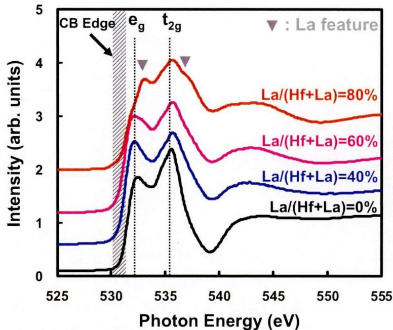
図5.16 HfLaO厚膜試料 [組成比: La/(Hf+La)= 0%, 40%, 60%, 80%]
