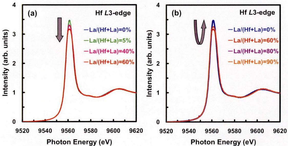
図 5.6 HfLaO 膜の Hf  $L_3$  XANES スペクトル; (a): La/(La+Hf)=0%, 5%, 40%, 60%, (b): La/(La+Hf)=0%, 60%, 80%, 90%.
