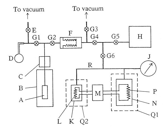
Fig. 4-4. Block diagram of the high pressure system. (A) Sample cell, (B) cryostat, (C) volume measurement system, (D) glass bulb, (E) PTFE cock, (F) pressure-transmitting-liquid separator, (G) high-pressure valves, (H) pressure generator, (J) Heise pressure gauge, (K) pressure sensor vessel, (L) Manganin pressure sensor, (M) pressure control circuit, (N) kerosene reservoir, (P) heater wire, (Q) thermostats, (R) pressure transmitting tubes.
