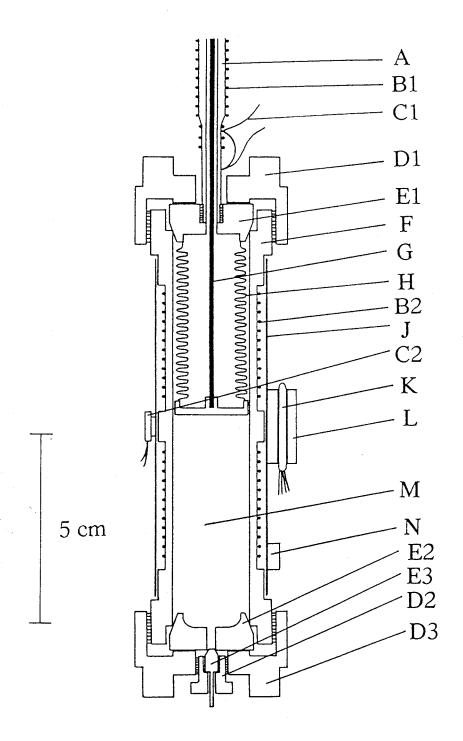
Fig. 4-2. Sectional drawing of the sample cell. (A) Pressure transmitting tube, (B) heater wires, (C) thermocouples, (D) gland nuts, (E) plugs, (F) main body of the cell, (G) displacement transmitting rod, (H) bellows, (J) cell cover, (K) Rh-Fe resistance thermometer, (L) thermometer holder, (M) sample room, (N) thermal anchor.
