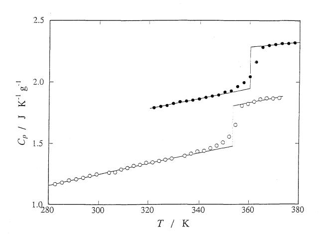
Fig. 5-1. Molar heat capacities of glassy and liquid atactic polystyrene at 0.1 MPa (open circles) and 21 MPa (closed circles). The data at 21 MPa are shifted upward by 0.5 JK<sup>-1</sup>g<sup>-1</sup> for the sake of clarity. The solid straight lines represent the extrapolations of the data used for the determination of  $\Delta C_p$  at  $T_g$ .
