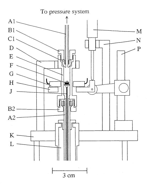
Fig. 4-3. Schematic drawing of the volume measurement system. (A) Pressure transmitting tubes, (B) gland nuts, (C) plugs, (D) supporting arm, (E) diamagnetic cylinder, (F) magnet, (G) Magnesensors, (H) Magnesensor holder, (J) displacement transmitting rod, (K) volume measurement stage, (L) cryostat, (M) Magnescale, (N) Magnescale holder, (P) cathetometer.
