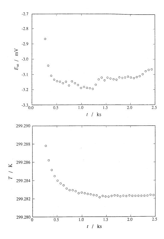
Fig. 4-17 Output signal of Magnesensor (upper) and the temperature of the cell (lower) measured after the energy input for the heat capacity and volume measurement.
