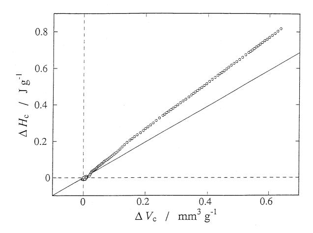
Fig. 6-2. Relaxation path of glassy atactic polystyrene in the  $\Delta H_{\rm C}$ - $\Delta V_{\rm C}$  plane. The solid line represents the equilibrium line.
