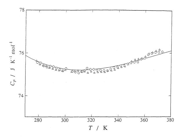
Fig. 4-11. Molar heat capacities of water. Circles and triangles denote the data in series 1 and 2, respectively. The solid line represents the literature smoothed curve [3].
