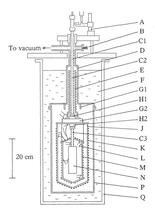
Fig. 4-1. Schematic drawing of the cryostat. (A) Volume measurement system, (B) flange for lead wires, (C1-C3) pressure transmitting tubes, (D) pumping tube, (E) adiabatic shield for the tube C2, (F) refrigerant, (G1,G2) thermal anchors, (H1,H2) couplings, (J) outer adiabatic shield, (K) heater wires, (L) thermocouples, (M) inner adiabatic shield, (N) sample cell, (P) vacuum jacket, (Q) Dewar flask.
