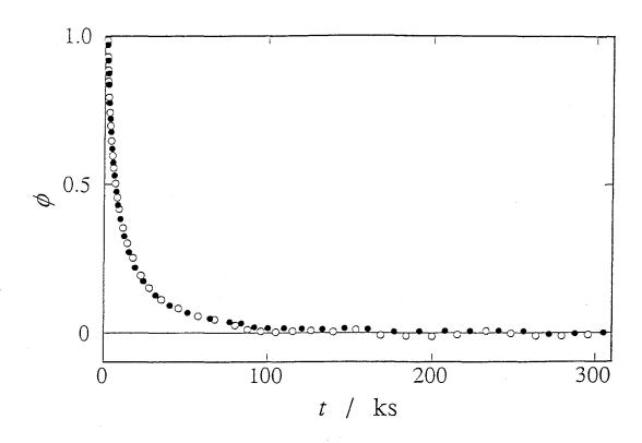
Fig. 6-1. Relaxation functions of glassy atactic polystyrene for the configurational enthalpy (open circles) and volume (closed circles) relaxations measured simultaneously.
