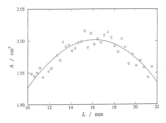
Fig. 4-10. Effective cross-sectional area of the bellows against its displacement.
