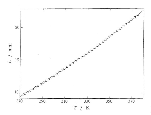
Fig. 4-8. Temperature dependence of the displacement of the bellows in the volume measurement of toluene.
