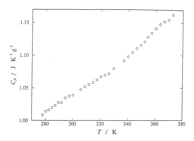
Fig. 4-13. Heat capacity of Fluorinert FC40.
