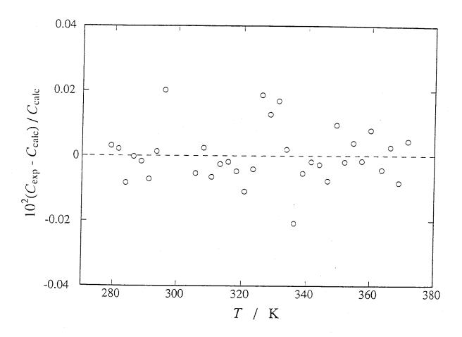
Fig. 4-6. Deviation plot of the observed heat capacities of the empty cell.
