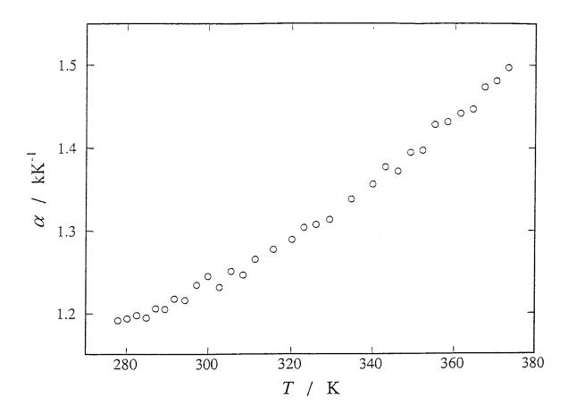
Fig. 4-15. Thermal expansivity of Fluorinert FC40.
