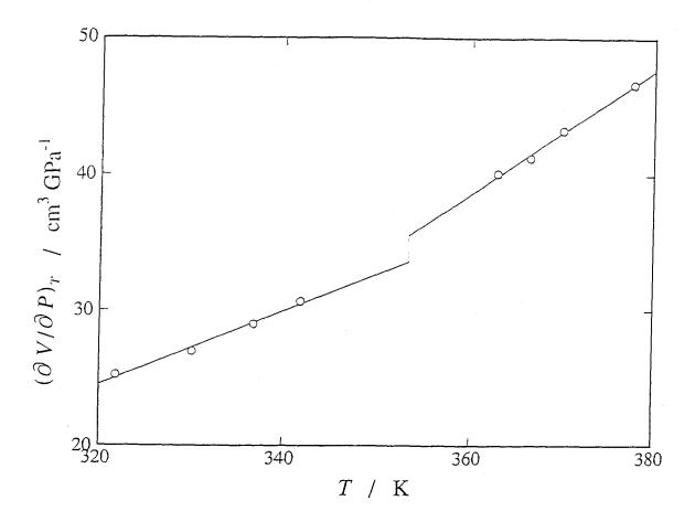
Fig. 5-3. Temperature dependence of  $(\partial V/\partial P)_T$  of atactic polystyrene at 0.1 MPa. The data contain the contributions from the sample, Fluorinert and the sample cup. The solid straight lines represent the extrapolations of the data used for the determination of  $\Delta \varkappa$  at  $T_g$ .
