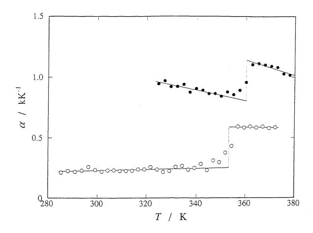
Fig. 5-2. Thermal expansivities of glassy and liquid atactic polystyrene at 0.1 MPa (open circles) and 21 MPa (closed circles). The data at 21 MPa are shifted upward by 0.5 kK<sup>-1</sup> for the sake of clarity. The solid straight lines represent the extrapolations of the data used for the determination of  $\Delta \alpha$  at  $T_g$ .
