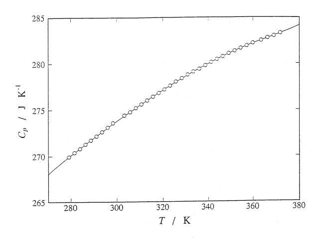
Fig. 4-5. Heat capacity of the empty cell. Solid line represents the curve smoothed by the least-squares fit.
