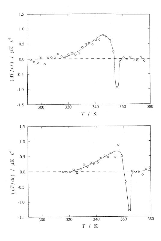
Fig. 5-4. Spontaneous temperature drift rates recorded during the heat capacity measurement of atactic polystyrene at 0.1 MPa (upper) and 21 MPa (lower).
