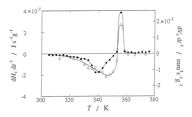
Fig. 5-5. Temperature dependence of the drift rates of configurational enthalpy (open circles) and volume (closed circles) in the simultaneous measurement of atactic polystyrene.
