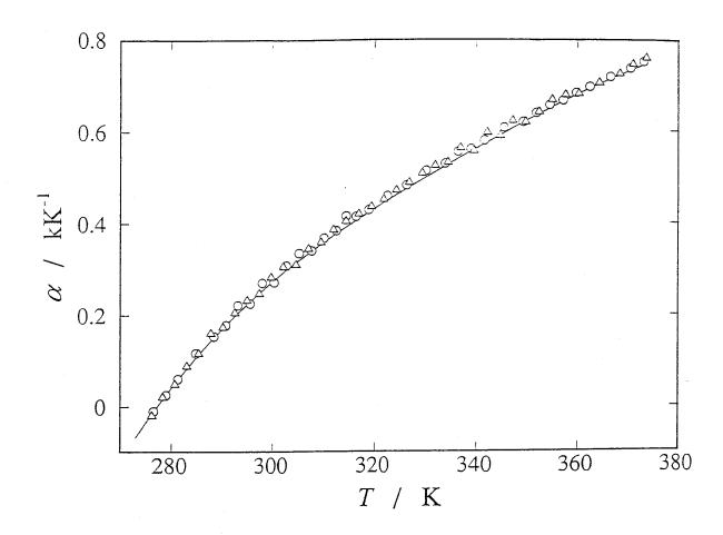
Fig. 4-12. Thermal expansivities of water. Circles and triangles denote the data in series 1 and 2, respectively. The solid line was calculated from the literature volume data [4].
