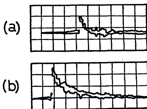
Fig.4-3 Oscilloscope traces of fluorescence decay curves of 9-9'-dianthryl, (a) in n-hexane, (b) in ethylalcohol.
