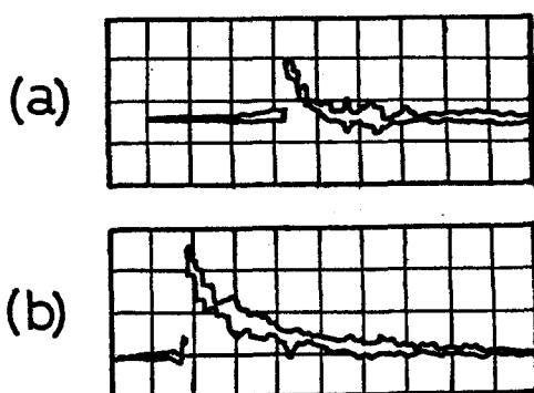
Fig. 4-3 Oscilloscope traces of fluorescence decay curves of 9-9'-dianthryl, (a) in n-hexane, (b) in ethylalchol.
