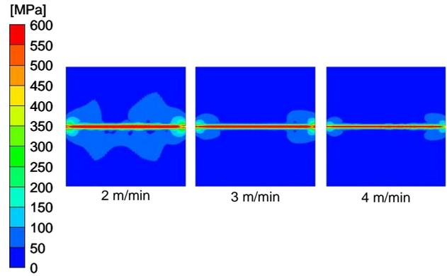
**Fig. 14** Effect of welding speed on von Mises residual stress after releasing fixtures.
