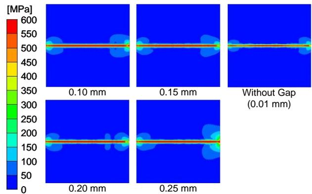
**Fig. 9** Effect of gap width on von Mises residual stress after releasing fixtures.
