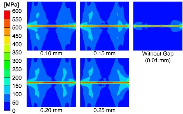
**Fig. 8** Effect of gap width on von Mises residual stress before releasing fixtures.
