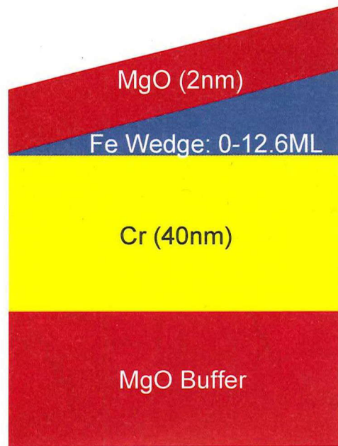
Fig.3.8 Sample structure for MOKE measurement
