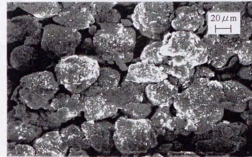
Fig.5-4 焼結体の微構造 Ni-Al 2 O 3 (14mass%,MF1),1373K
