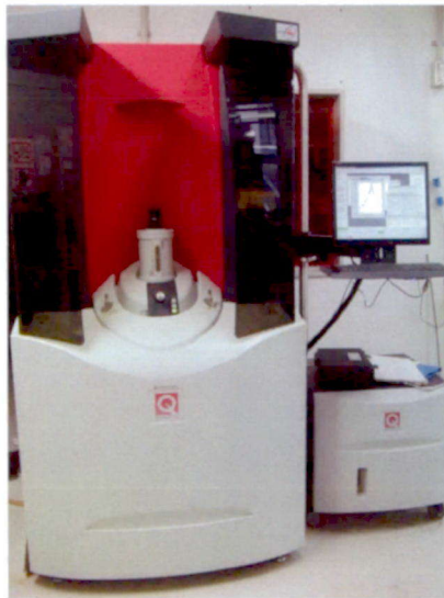
Figure 2.4. A picture of the VSM-SQUID
