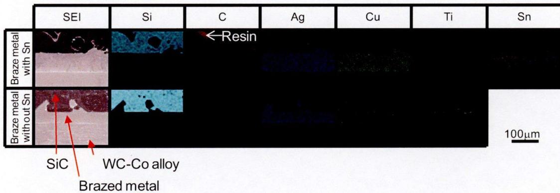
Fig. 4.8 Secondary electron image (SEI) and element distributions of Si, C, Ag, Cu, Ti and Sn at cross-sections of brazed joints of silicon carbide and WC-Co alloy using braze metals with and without Sn.
