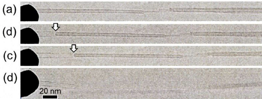
Fig. 5.1 Series of TEM images for an extraction process. (a) Two CNTs with sharpened tips are in contact. (b), (c) Left side inner shell is extracted following the right side CNT. White arrows indicate the ends of the inner shell. (d) Left side inner shell is extracted completely and the outer several layers remain at the left-side electrode.
