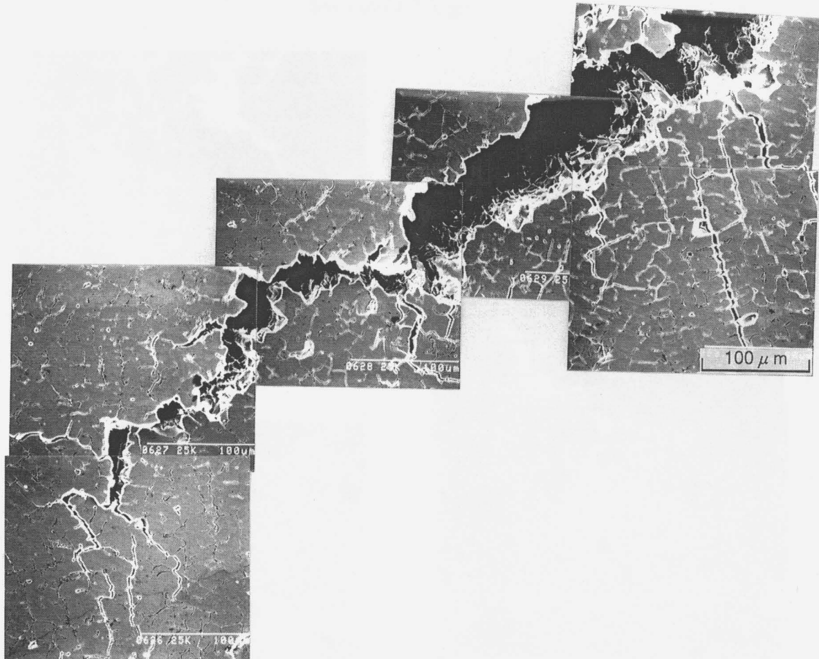
(f) Tip of crack
