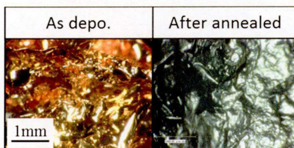
Fig. 6.2 Visual picture of Cu after TG-DTA.
