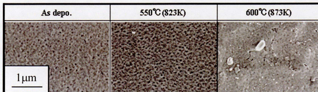
Fig. 3.24 Surface observation of Glass/ \text{Cr}_2\text{O}_3 /Cr/Cu/Cr/ \text{SnO}_2 by FE-SEM.
