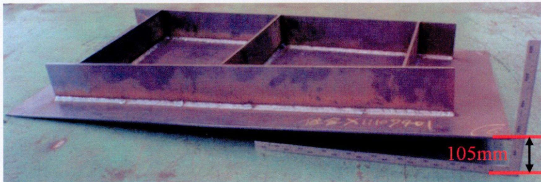
Fig. 6.3 Deformed shape of welded structure after welding.
