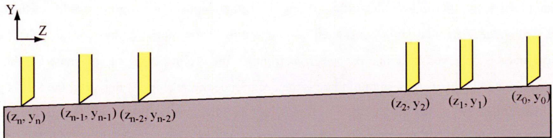
Fig. 2-23 Method to calculate the inclination of workpiece
