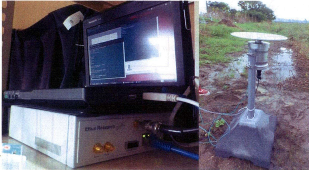
Figure 2.6 Main components of a single station of LF lightning location system.
