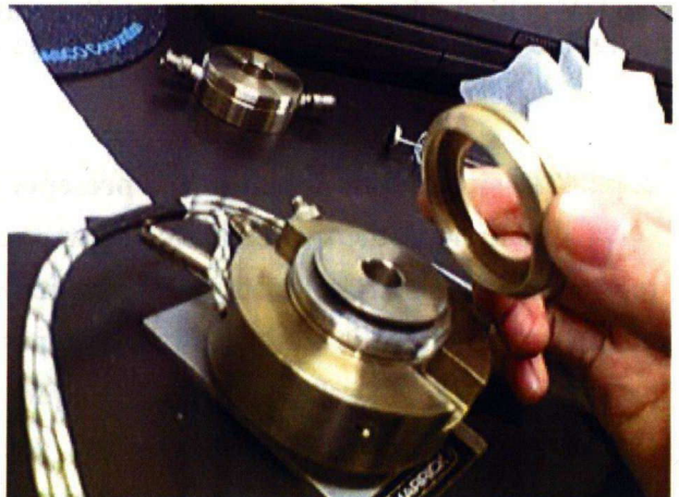
Figure 2.2.3. The photographs for the experimental setting up of the in-situ UV cell.
