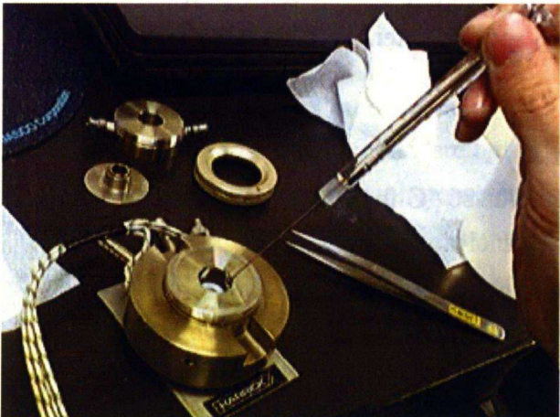
Figure 2.2.3. The photographs for the experimental setting up of the in-situ UV cell.
