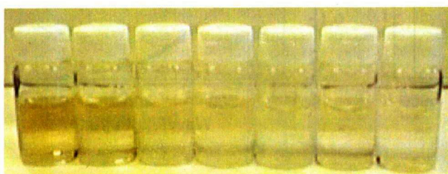
Fig. 3.2.3. Color changes of Nordic fulvic acid solution (100mg/L) at 180°C for 0 - 18 hours.
